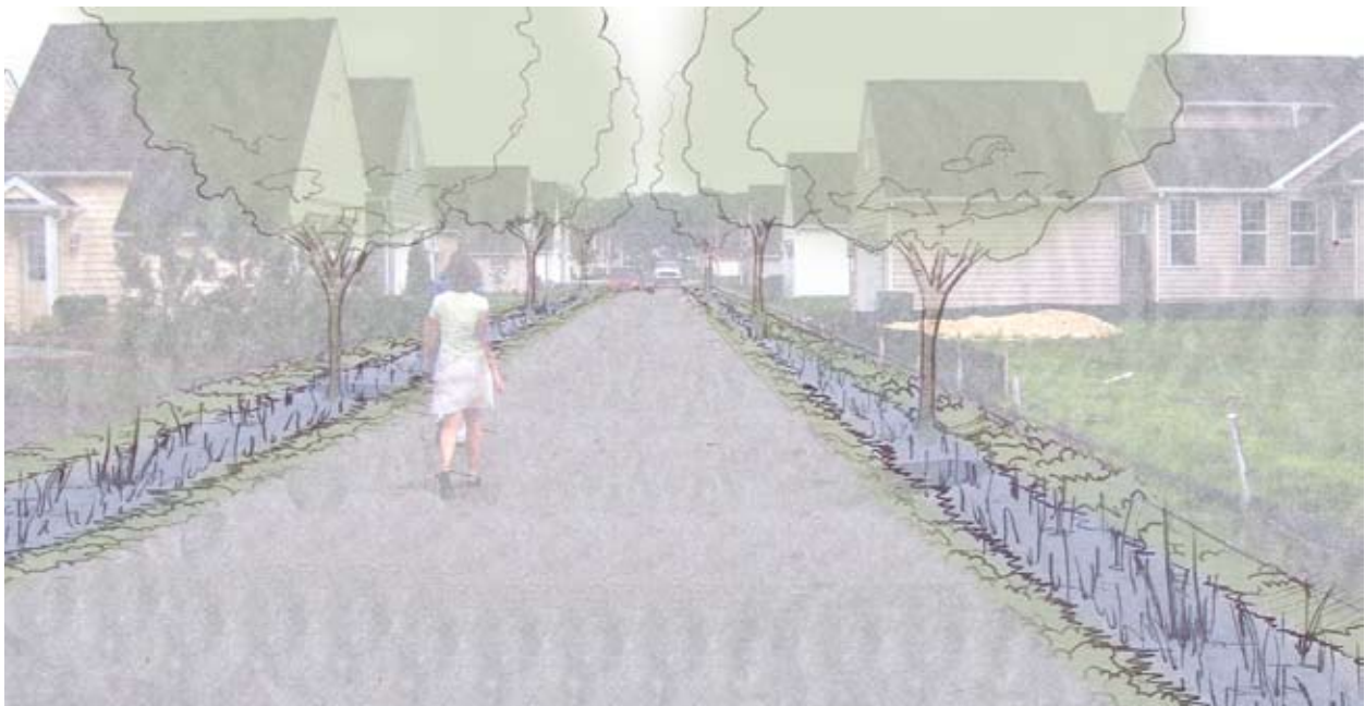
Figure 5-23: RETROFIT OPPORTUNITY: Same residential alley retrofitted with side stormwater swales.
