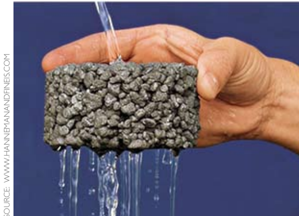
Figure 4-15: Pervious concrete allows water to pass through pore spaces in the aggregate.
