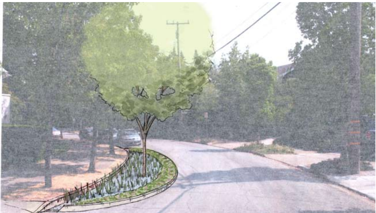
Figure 5-11: RETROFIT OPPORTUNITY: Same residential street retrofitted with mid-block stormwater curb extensions as well as additional street trees.
