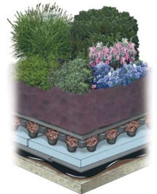
Figure 4-5: Typical profile for an intensive green roof system.
