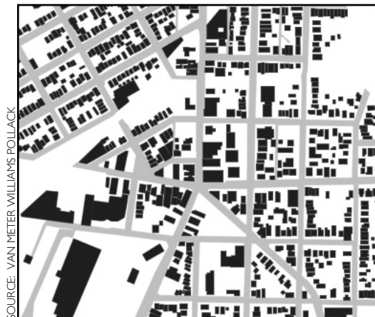
Figure 3-2: The shaded areas in this diagram represent the impervious area associated with streets and buildings in the same neighborhood represented in Figure 3-1.
