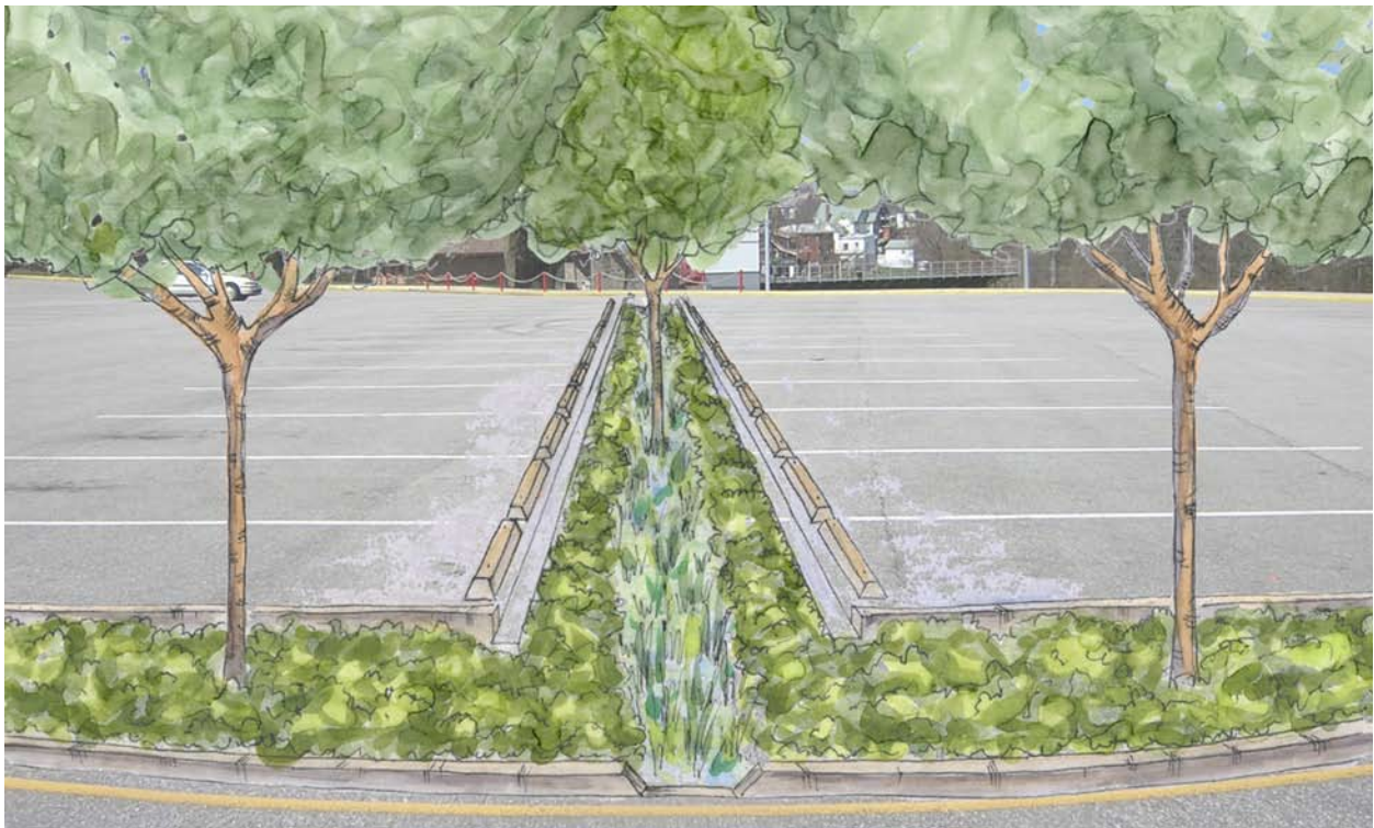
Figure 5-67: RETROFIT OPPORTUNITY: Same parking lot retrofitted with a center median stormwater swale. Introducing this new landscaped area can help cool the parking lot surface and increase overall aesthetics.
