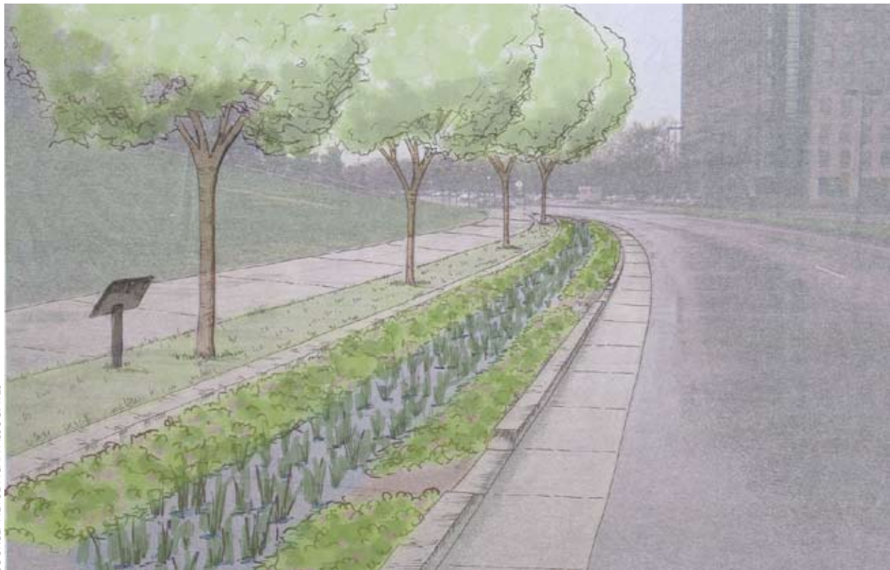
Figure 5-55: RETROFIT OPPORTUNITY: Same street consolidates the wide sidewalk space for a stormwater swale and street trees along the boulevard.
