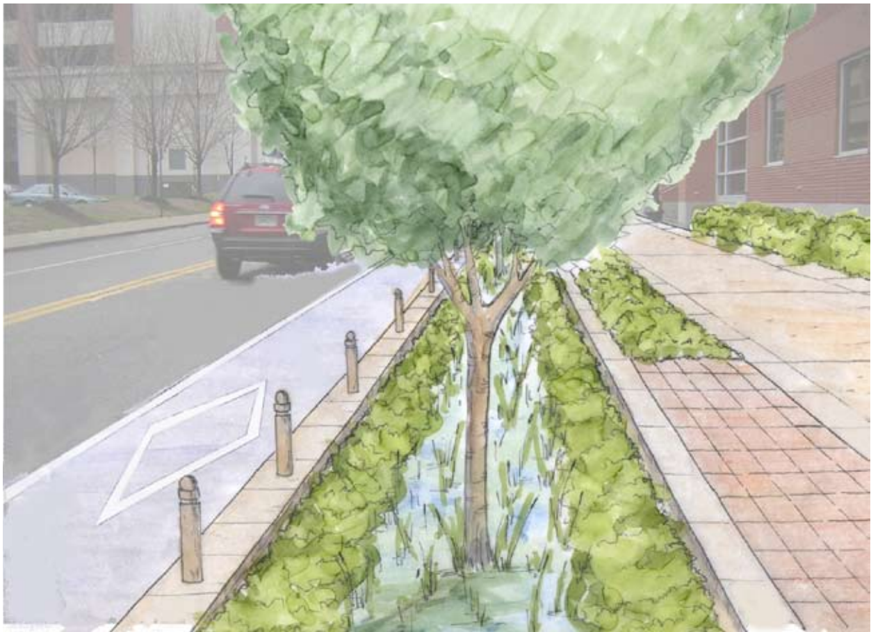
Figure 5-31: RETROFIT OPPORTUNITY: Same street without one traffic lane and retrofitted with a "curbless" street, vegetated swale, and bike lane.
