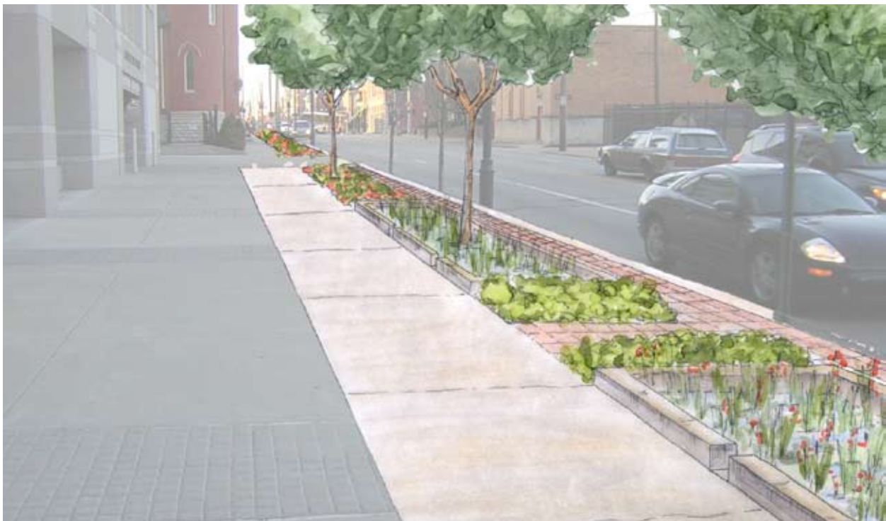
Figure 5-27: RETROFIT OPPORTUNITY: Same commercial street retrofitted with a series of stormwater planters.
