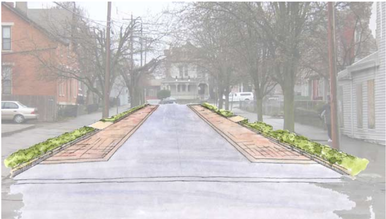
Figure 5-19: RETROFIT OPPORTUNITY: Same residential street retrofitted with pervious paving in the parking zone of the street.
