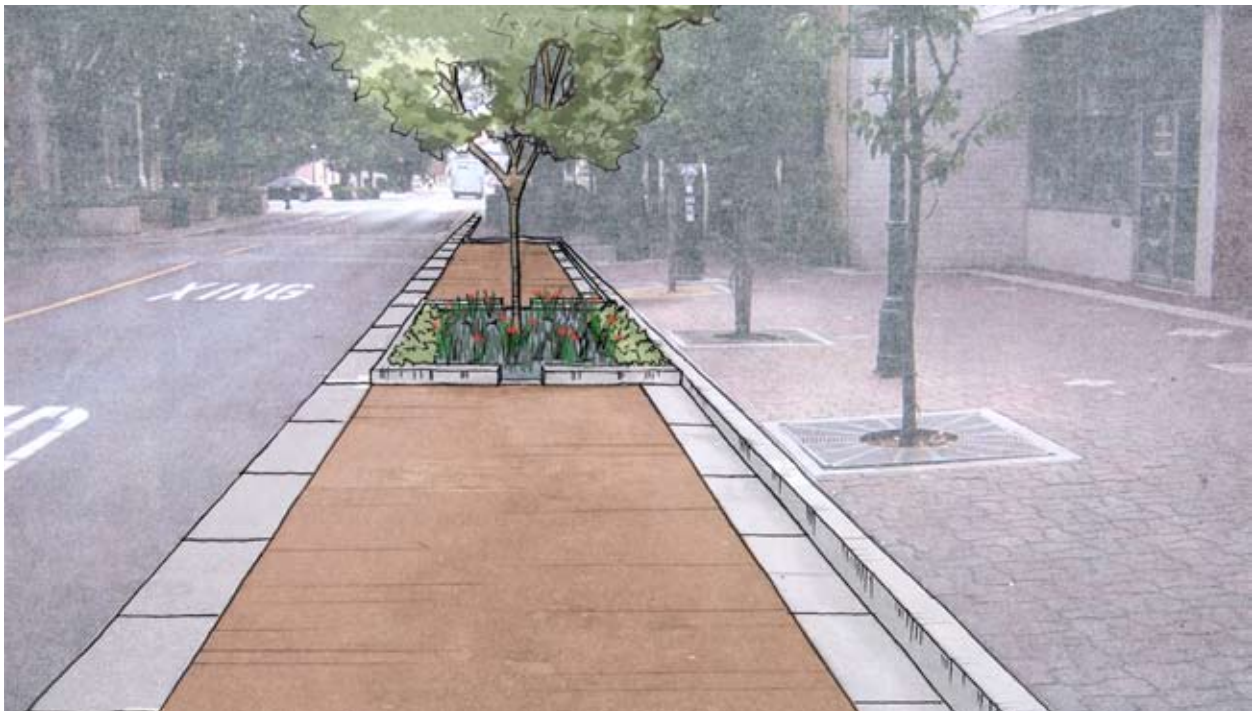
Figure 5-39: RETROFIT OPPORTUNITY: Same commercial street with pervious paving in the parking zone and stormwater curb extensions.
