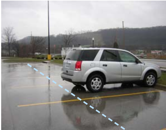
Figure 3-11: Shortening these oversized parking spaces by just a few feet could create space for swales.
