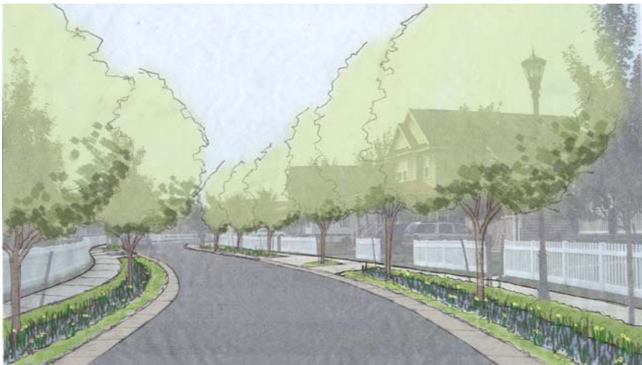
Figure 5-15: RETROFIT OPPORTUNITY: Same residential street using vegetated swales in the street's planting strips.
