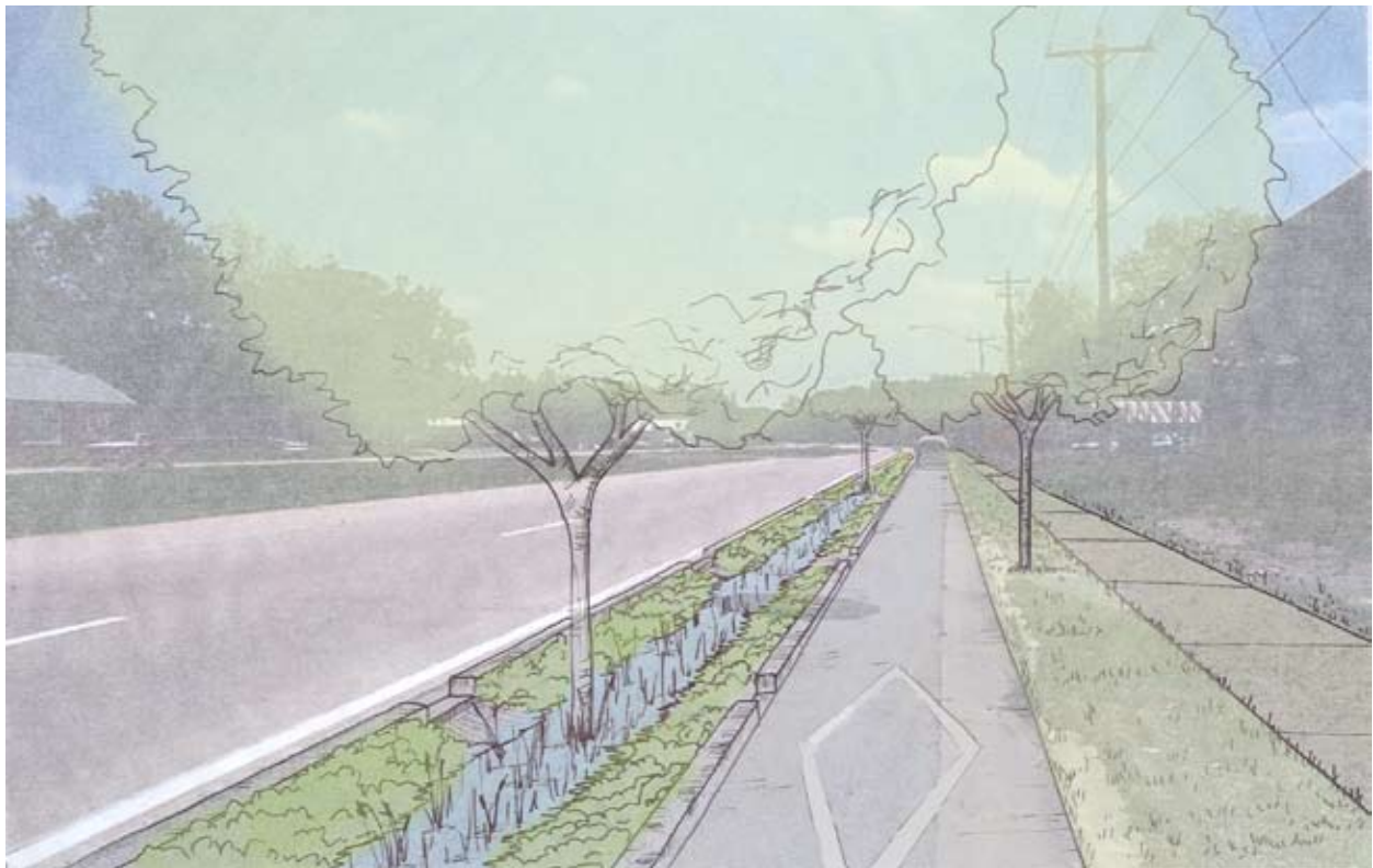
Figure 5-53: RETROFIT OPPORTUNITY: This retrofit example meets multiple goals by adding a bike lane that is buffered from the road, a sidewalk, and a stormwater swale.
