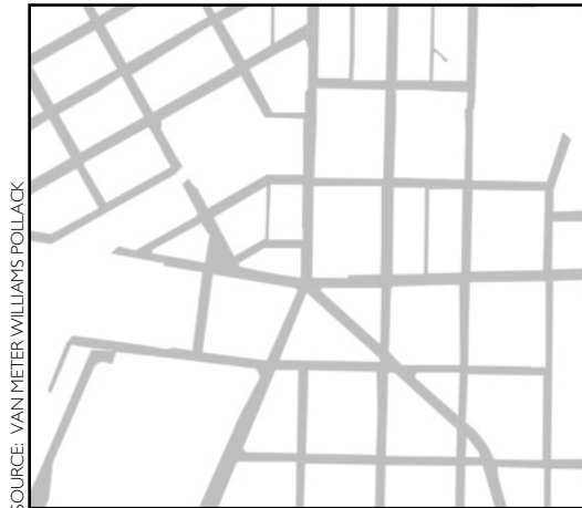
Figure 3-1: The shaded areas in this diagram represent the impervious area associated with streets.
