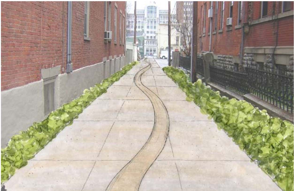
Figure 5-49: RETROFIT OPPORTUNITY: Same alley retrofitted with pervious concrete and an artistic valley gutter to convey overflow.
