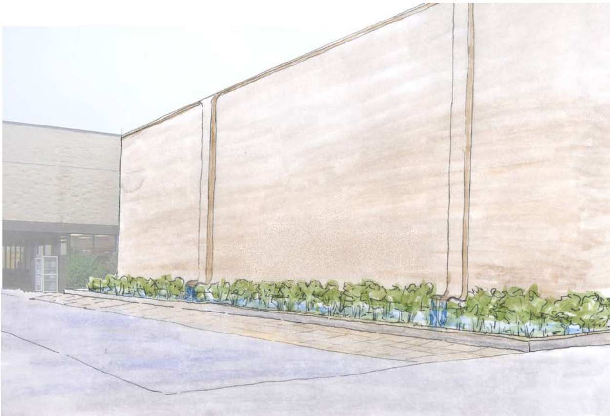
Figure 5-78: RETROFIT OPPORTUNITY: Same store retrofitted with a stormwater planter in the existing foundation planting space.
