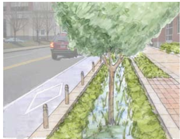
Figure 3-8: The same street redesigned to accommodate a new bike lane, enhanced landscaping, and stormwater management.
