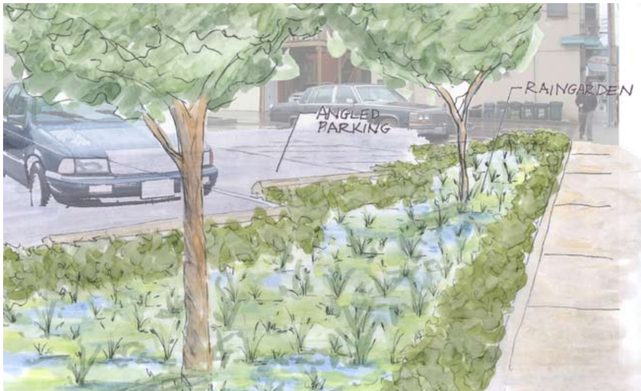
Figure 5-63: RETROFIT OPPORTUNITY: Same parking lot retrofitted with a stormwater swale/planter.
