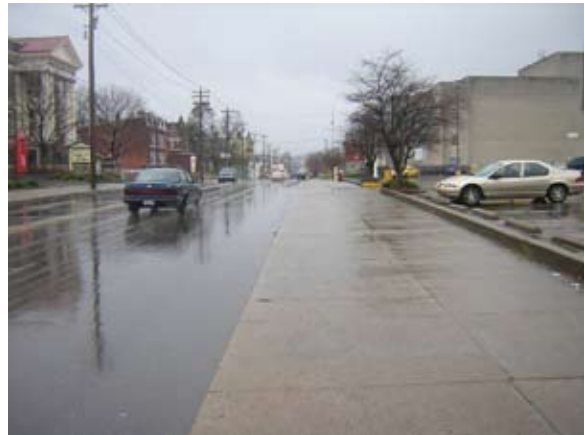
Figure 5-46: EXISTING: A typical urban street in Northern Kentucky with no on-street parking. The travel lane and sidewalk are twice as wide as needed.
