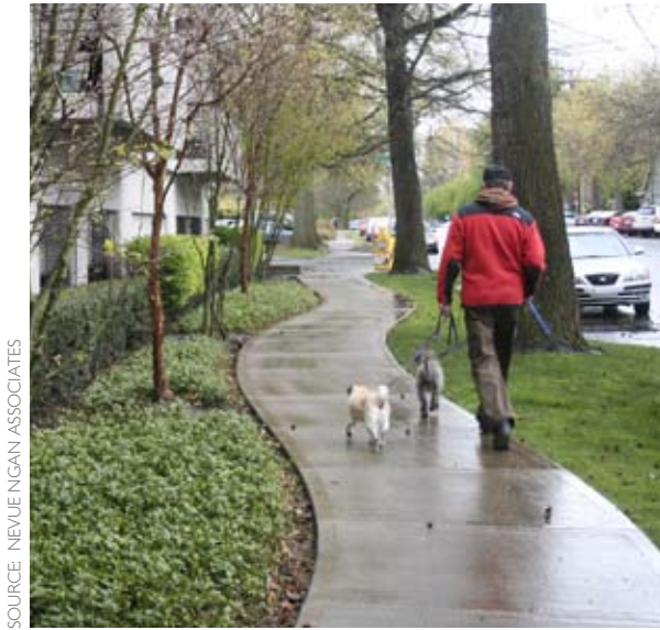
Figure F-1: These mature street trees were saved by allowing the sidewalk to curve around the trees. However, the new sidewalk alignment also reduced the size of the adjacent stormwater swale.
