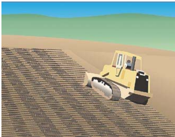
Tread-track slopes up and down hill to improve stability.
