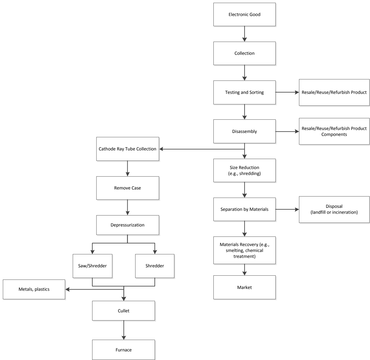
Figure 5-4: Electronics Recycling Process
