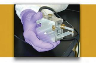
"EPA researchers have developed an improved, cost-effective instrument for measuring the thickness of soft biological tissues."
