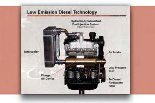
"The innovative design allows an average fuel economy improvement of 30 to 40 percent over gasoline engines and produces the lowest known engine-out NOx ever achieved by any diesel engine."
