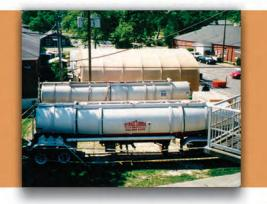
"The pervaporation system provides a sustainable method of removing VOCs from groundwater, soil-washing and soil-flushing solutions, and industrial waste streams."
