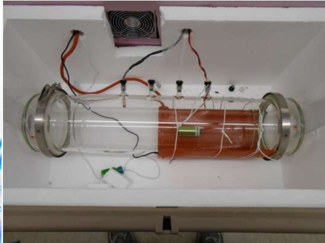
CairClip electrochemical sensor evaluated under the Air Sensors Project
