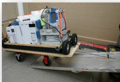
Figure 3: Loading the GC/MS into the mobile lab
