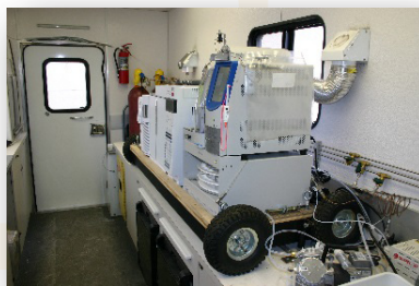
Figure 2: Trailer Mounted GC/MS System
