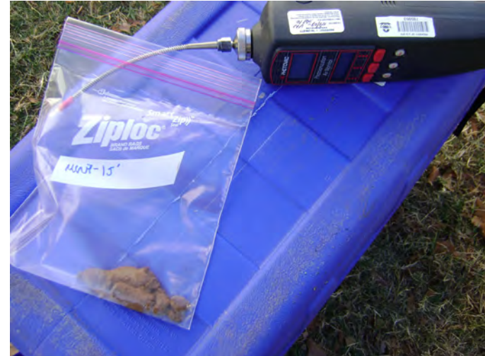
Figure A-6. After the volatile hydrocarbons in the subsample equilibrated with the air in the sealed plastic bag, the concentration of hydrocarbons were measured with an organic vapor meter.
