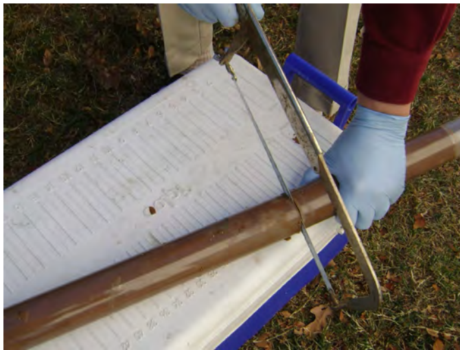
Figure A-3. A core sample acquired in a plastic sleeve is cut to access the core for sub sampling.
