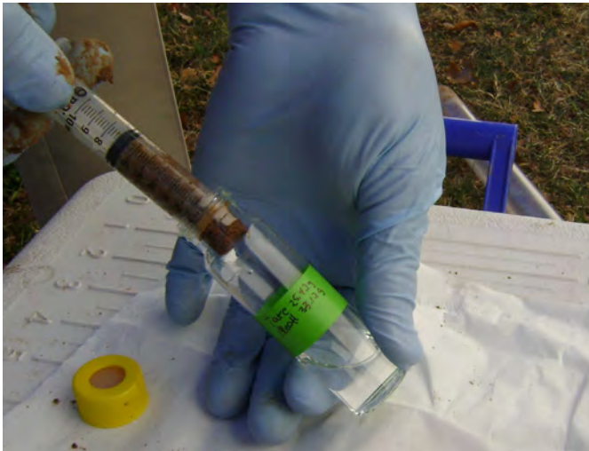
Figure A-7. Each subsample for analysis in the laboratory is introduced into a vial previously prepared with 10 ml of methanol
