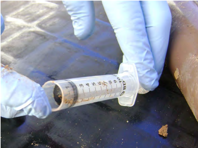
Figure A-1. A sampler was constructed by cutting the end out of a plastic syringe.
