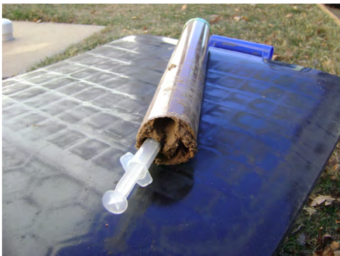
Figure A-5. Additional samples are acquired from the cut face as needed. One sample is transferred to a plastic bag for screening of volatile organic hydrocarbons. See Figure A-6.
