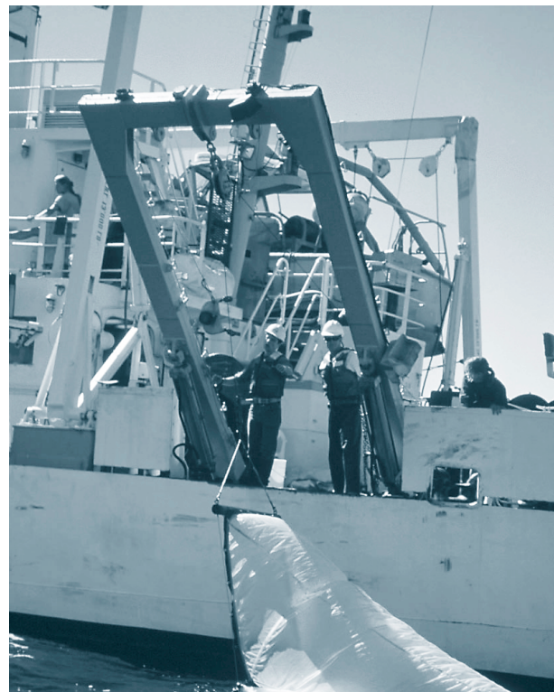
Scientists retrieve a Tucker net, which has three nets to sample different depths and obtain discrete samples of tiny organisms that make up the base of the food web in the Cordell Bank Sanctuary (Photo: Jamie Hall).
