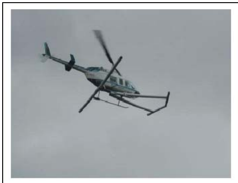
Figure 9-3. Airborne Geophysical Survey Helicopter Platform (from Oak Ridge National Laboratory, 2002).
