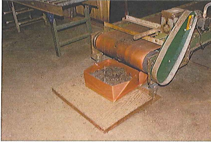
Tritonal Flaking Belt – Building 1619
