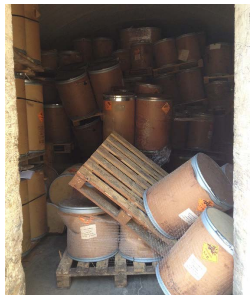
Photo 12: M6 and Tritonal/Aluminum/TNT containers falling and spilling contents inside magazines
