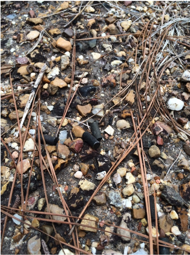
Photo 7: M6 Propellant spilled outside magazines exposed to elements
