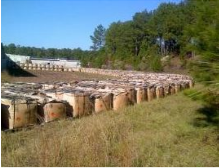
Photo 1: M6 Propellant improperly stored outside by Explo
