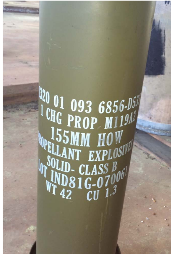
Photo 8: M119A2 155MM Propelling Charge provided to Explo by US Army for demilitarization; Origin of M6 Propellant
