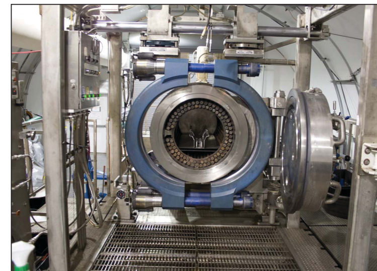
The Explosive Destruction System destroys recovered chemical warfare materiel while protecting workers and the environment.
