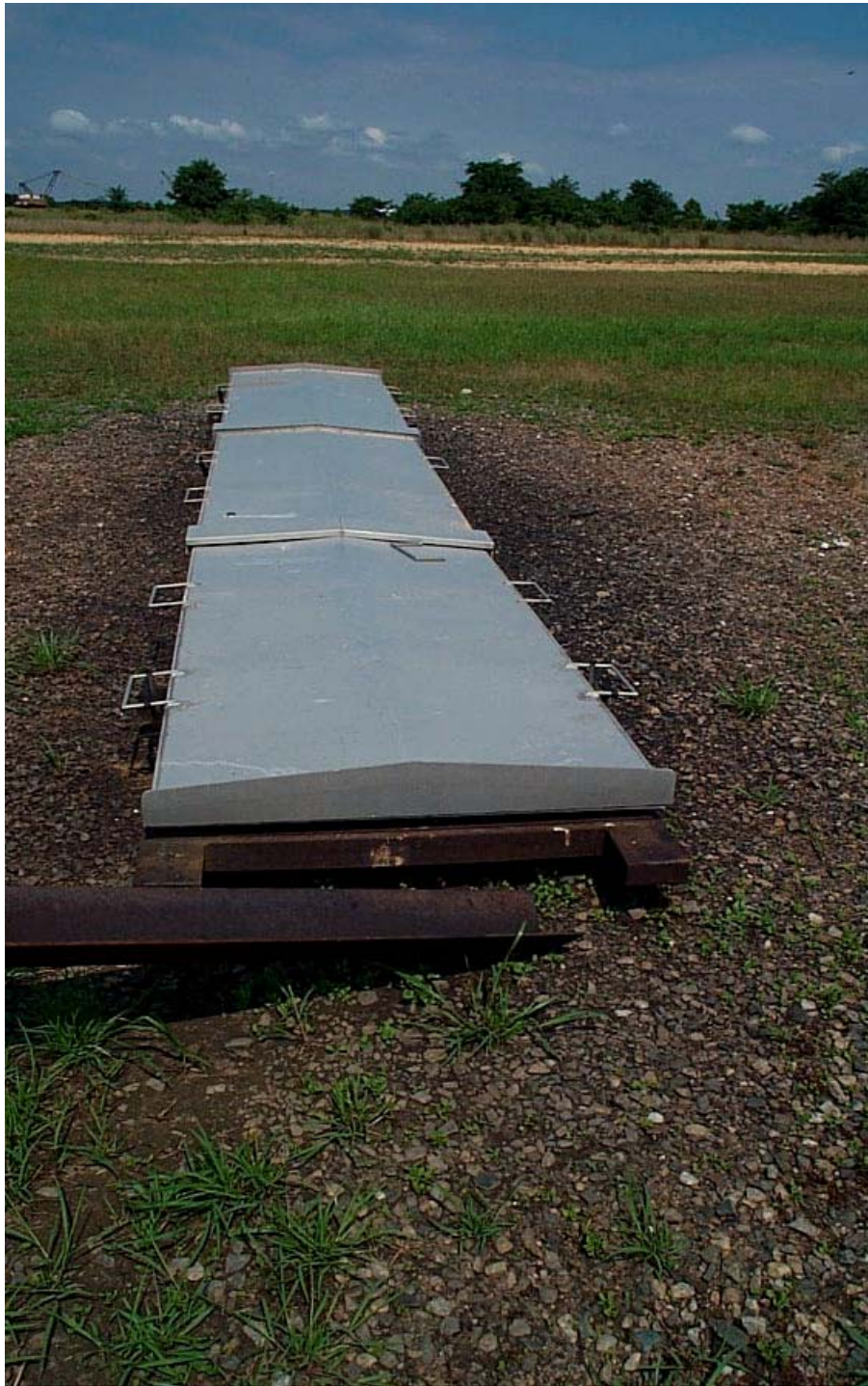
Fig. 2-2. Example burn pans with precipitation covers
