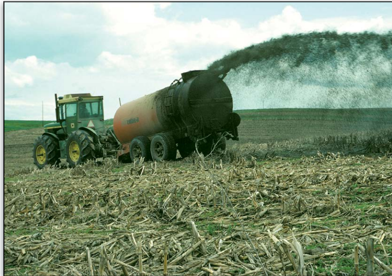
Liquid manure from a hog feeding operation in northeast Iowa is being pumped onto cropland with a honey wagon.
