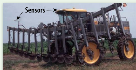
Hagie equipped with coulters and rigid injection of liquid urea ammonium nitrate. Adequate clearance ranges from 1.5 to about 5.5 feet.
