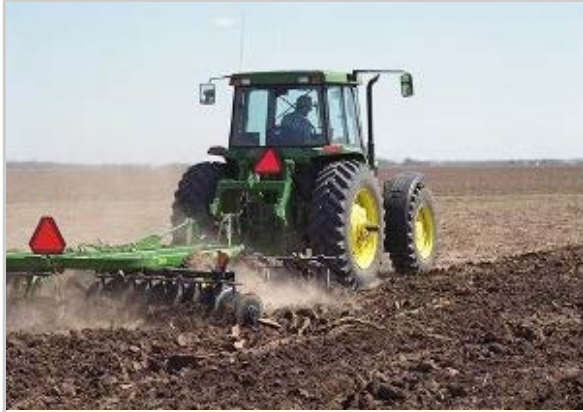
A field shot of a tractor and disk harrow at work Source: Deere Photo Library, Vol. 1
