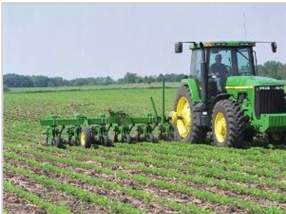
A tractor and row crop cultivator working in soybeans planted with a conservation tillage system Source: Deere Photo Library, Vol. 1
