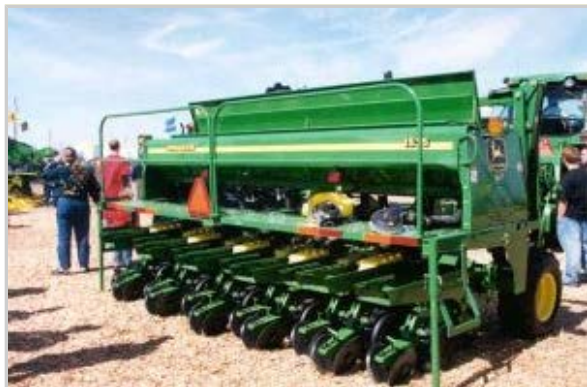
A grain drill on display at a farm machinery show Source: Daniel R. Ess, Purdue University
