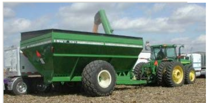
A large-capacity grain cart unloading into a waiting truck Source: Daniel R. Ess, Purdue University
