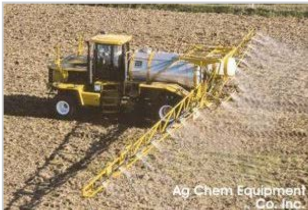
A self-propelled sprayer broadcasting crop chemicals in the field Source: Ag-Chem, a division of AGCO Corporation
