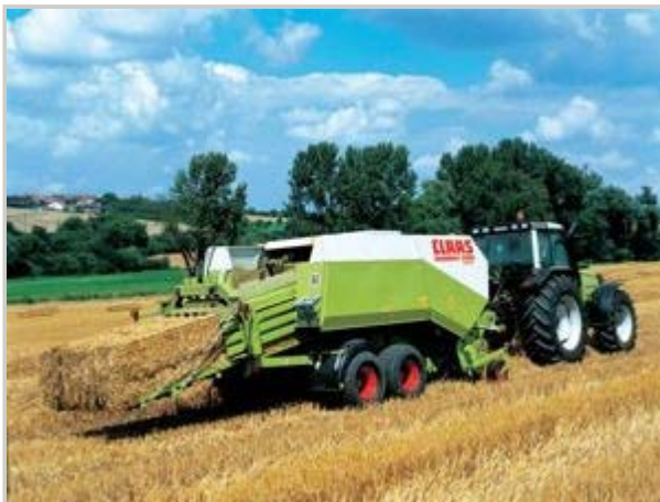
Large rectangular baler discharging a newly-formed bale of straw Source: Class of America
