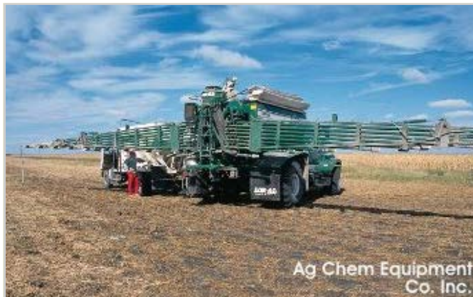
A self-propelled spreader that uses a pneumatic system to evenly distribute dry crop chemicals Source: Ag-Chem, a division of AGCO Corporation
