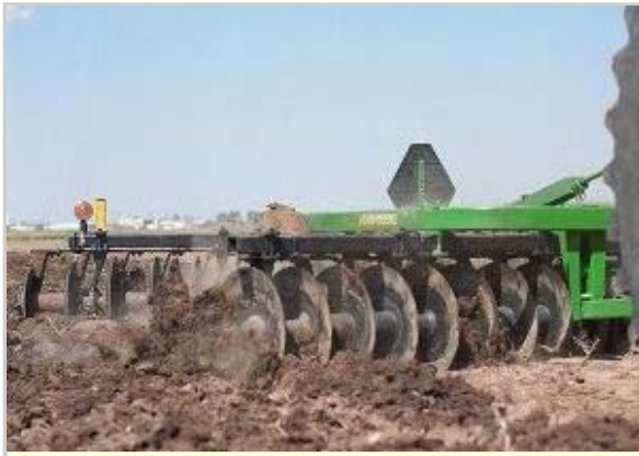
A close-up view of a disk harrow in the field Source: Deere Photo Library, Vol. 1
