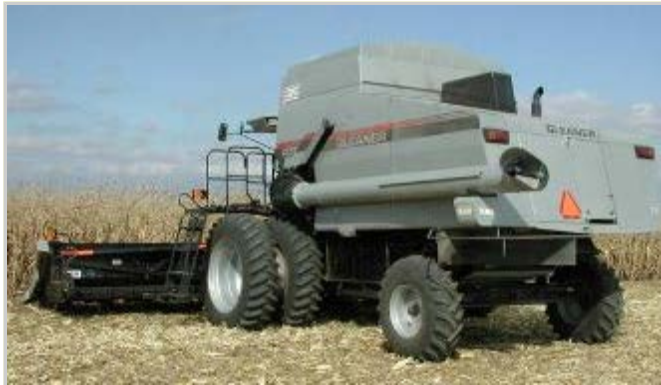
Self-propelled combine equipped with a corn head preparing to harvest corn Source: Daniel R. Ess, Purdue University
