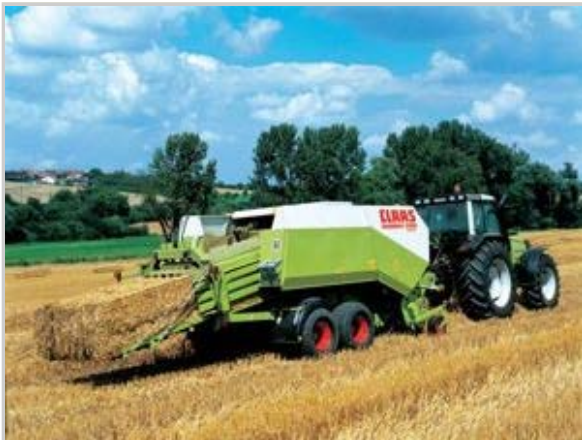
Large rectangular baler discharging a newly-formed bale of straw Source: Class of America
