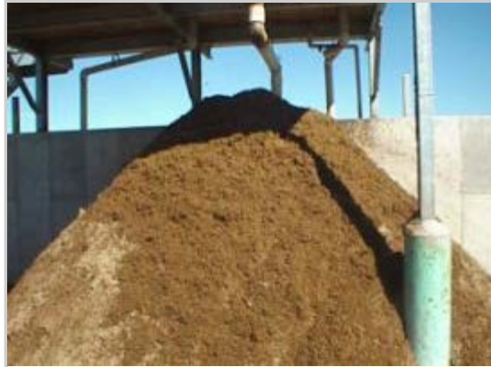
Effluent drips down for collection
