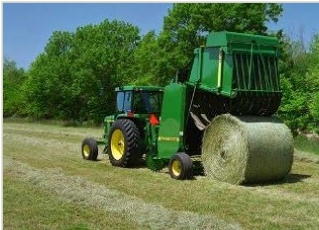
Large round baler discharging a newly-formed bale of hay Source: Deere Photo Library, Vol. 3
