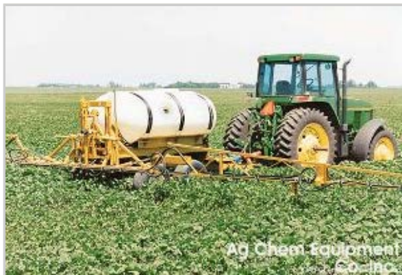
A pull-type sprayer and tractor Source: Ag-Chem, a division of AGCO Corporation
