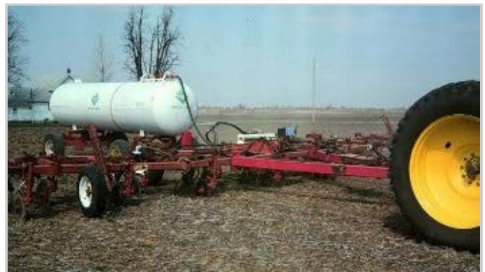
A tractor-drawn toolbar being used to inject anhydrous ammonia into the soil. The wagon mounted tank attached to the toolbar supplied ammonia. Source: Daniel R. Ess, Purdue University
