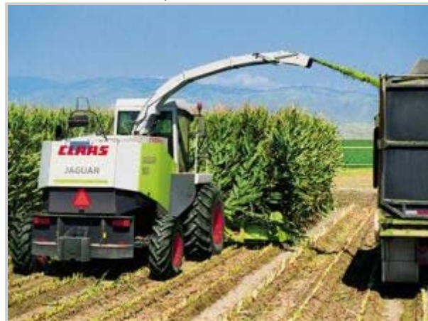
A self-propelled forage harvester loading chopped corn into a truck on-the-go. Source: Class of America
