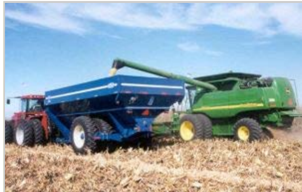
Harvest scene in the Corn Belt - a large combine quickly unloads grain to a high-capacity grain cart Source: Daniel R. Ess, Purdue University
