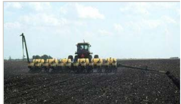
A twelve-row planter working in a conventionally-tilled field Source: Daniel R. Ess, Purdue University
