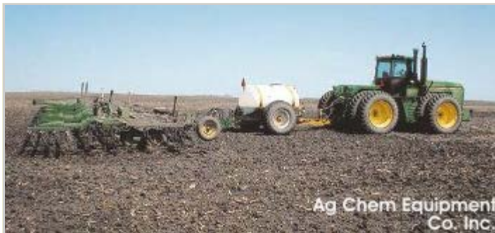
A tractor-sprayer-field cultivator combo that performs tillage and crop chemical application operations simultaneously Source: Ag-Chem, a division of AGCO Corporation
