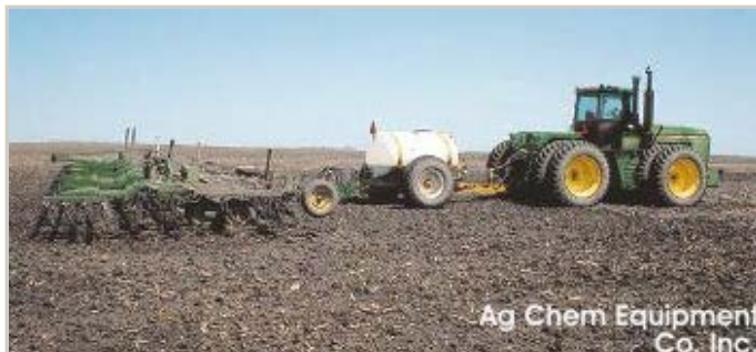
A tractor-sprayer-field cultivator combo that performs tillage and crop chemical application operations simultaneously
