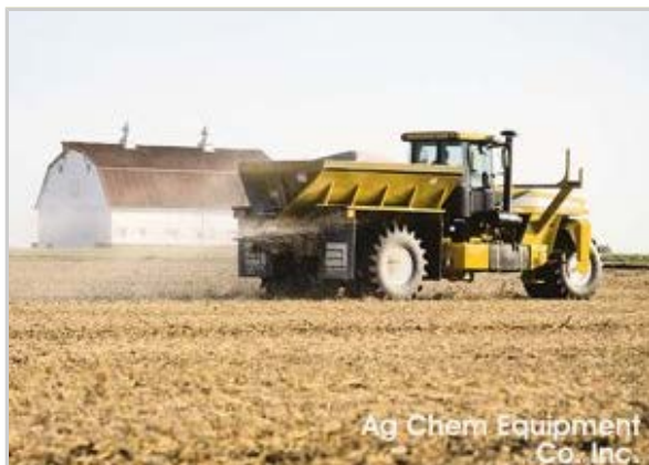
A self-propelled spreader that uses spinning disks to distribute dry crop chemicals Source: Ag-Chem, a division of AGCO Corporation
