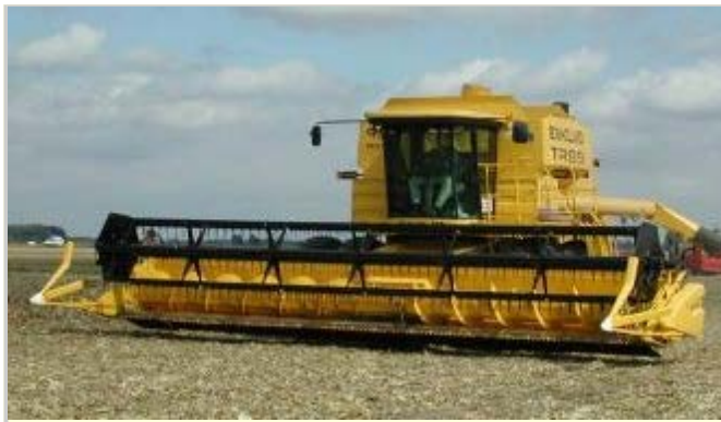
Self-propelled combine equipped with a grain header Source: Daniel R. Ess, Purdue University
