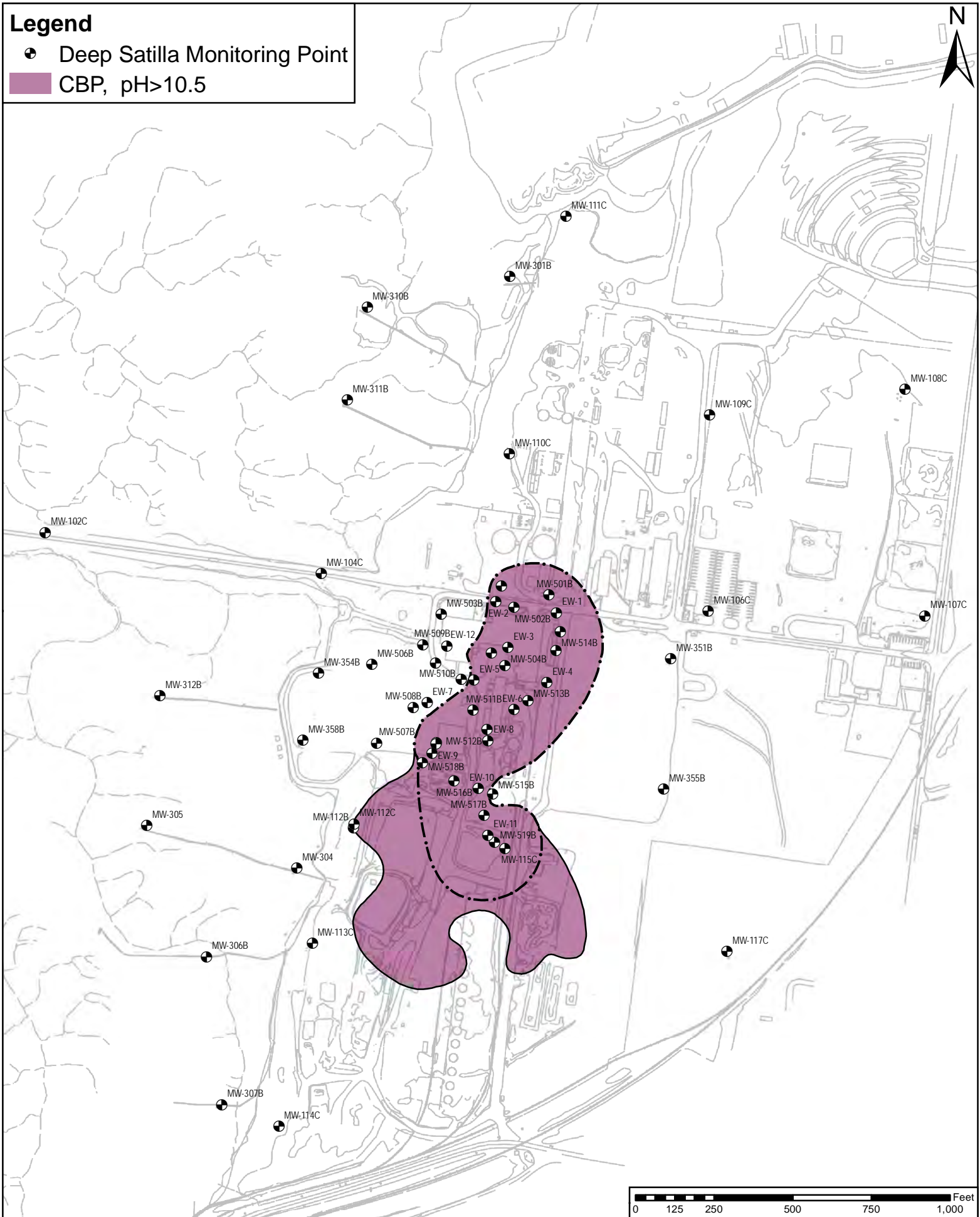
Figure 1-3: Updated location of the CBP using 2014 Geoprobe pH data. LCP Chemicals Site, Brunswick, GA
