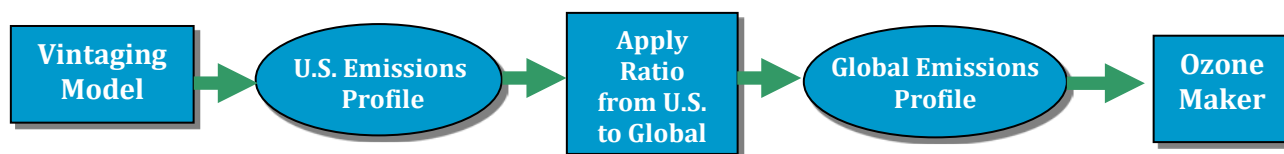
Figure 2: Schematic Diagram of Historical Method for Relating Emissions to Stratospheric Ozone Projections in the AHEF
