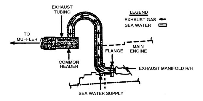
Figure 2. Typical Water Jacketed Elevated Loop<sup>12</sup>
