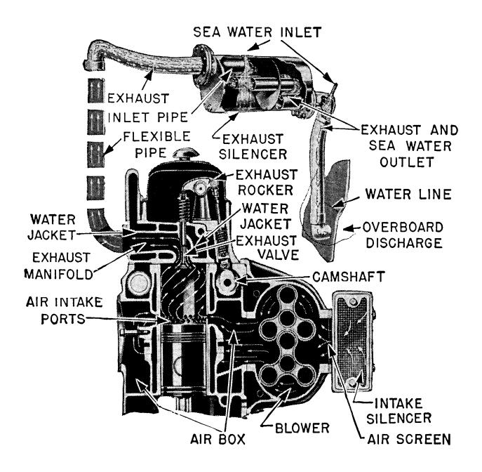
Figure 1. Air Systems of a Two-Stroke Cycle Engine (GM71)<sup>11</sup>
