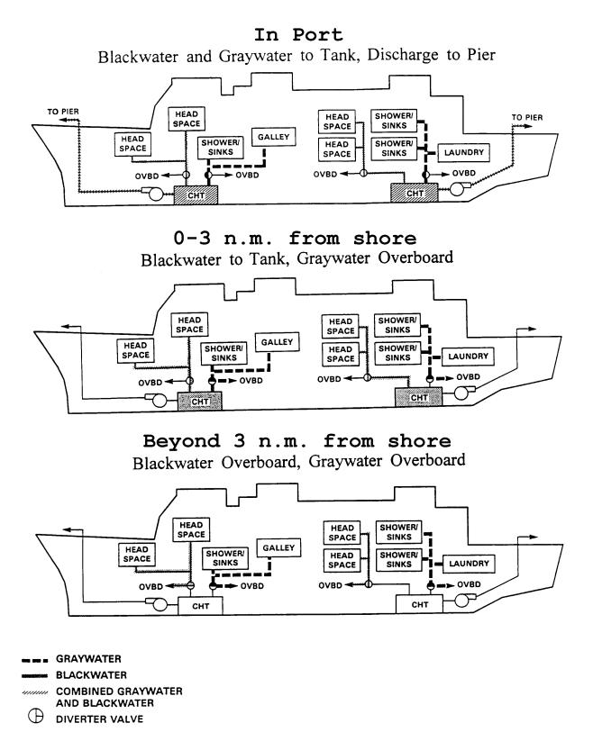
Figure 1. A Typical Collection, Holding, and Transfer System
