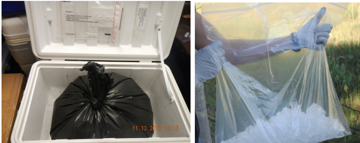
Figure 3-14. Samples in a Sealed Bag and Bags of Ice to Keep the Samples Cold During Shipping
