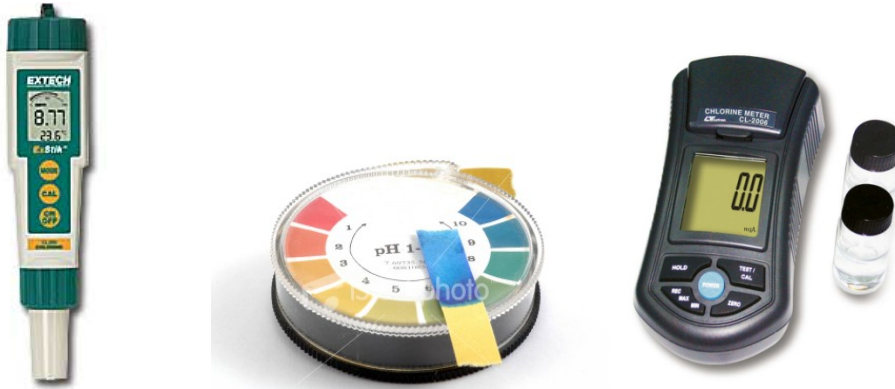
Figure 3-3. Typical Field Measurement Meters and Strips for Chlorine and pH.
