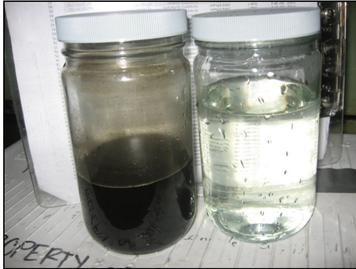
Figure 2-1. A Comparison of the Bilgewater Samples Taken Before and After Bilgewater Treatment
