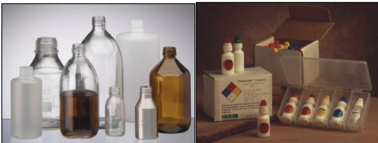
Figure 3-2. Example of Various Types of Sample Bottles and Various Preservation Chemicals in Dropper Bottles
