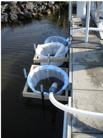
Photograph 27: Net Set-up With Hoses
