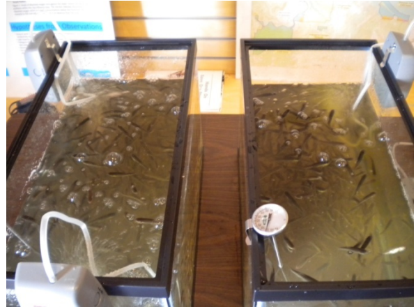
Photograph 20: Influent Tanks with Aerators and Thermometers
