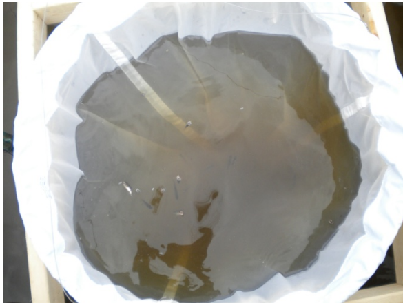
Photograph 39: Pump Effluent in Netting
