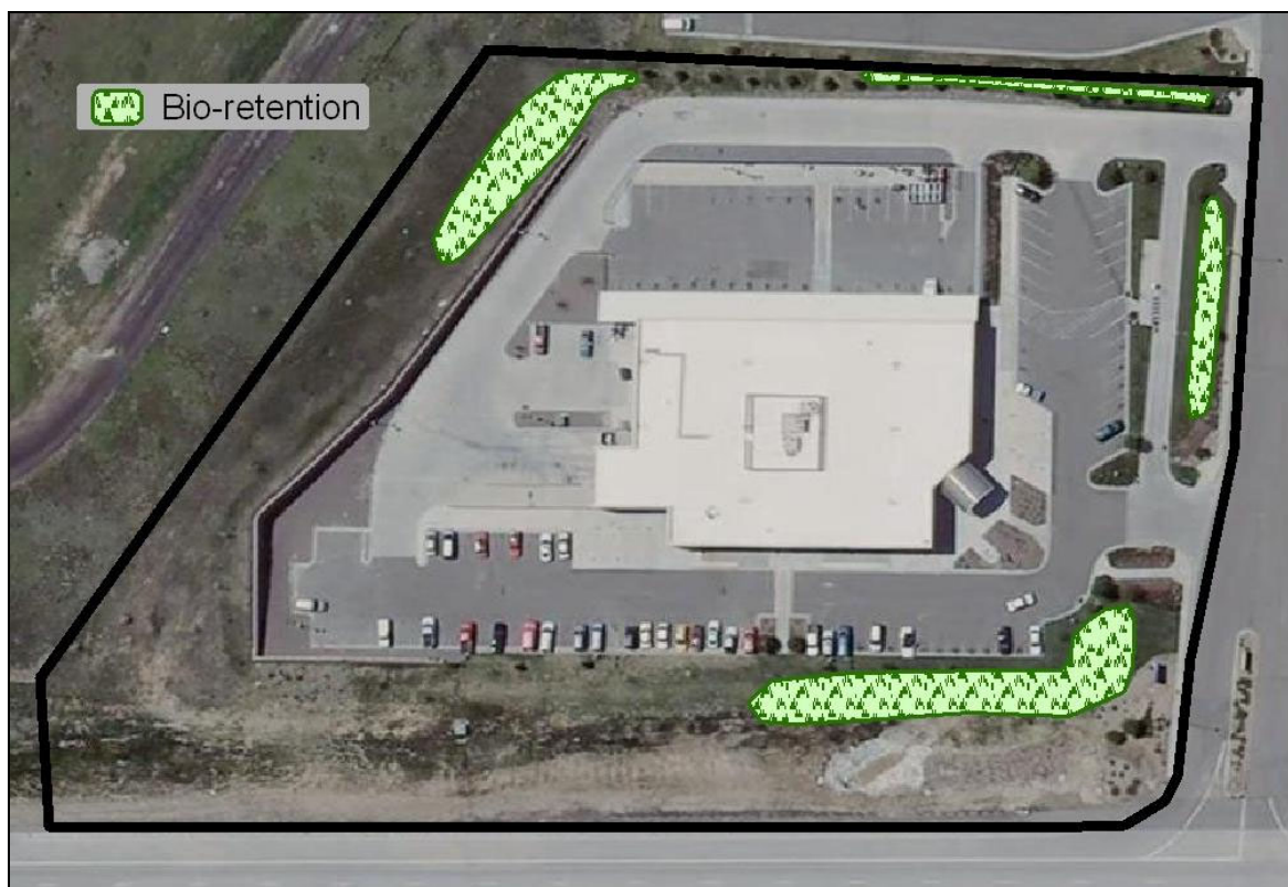
Figure 3A3-4. Actual site and on-site control measures (Denver, CO).
