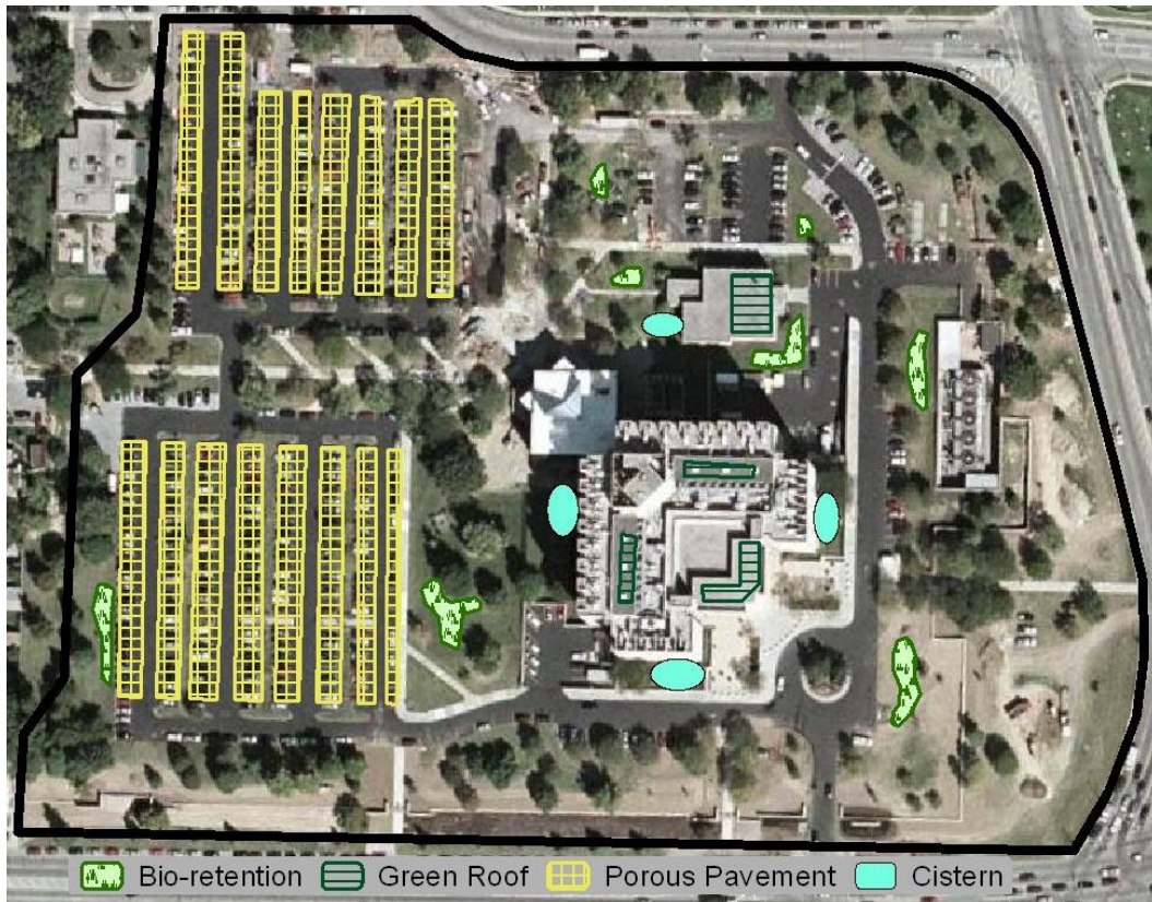
Figure 3A3-10. Actual site and on-site control measures (Cincinnati, OH).
