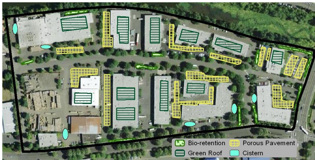
Figure 3A3-6. Actual site and onsite control measures (Portland, OR).
