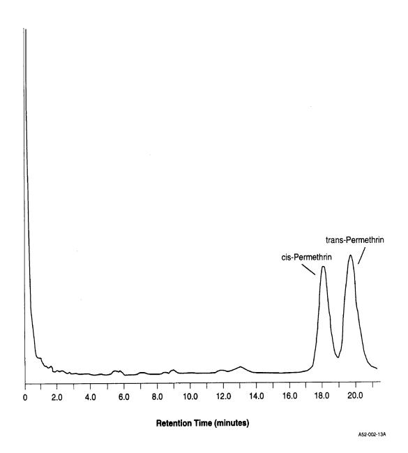
Figure 2. Gas Chromatogram of Permethrin Sample (Column 1)
