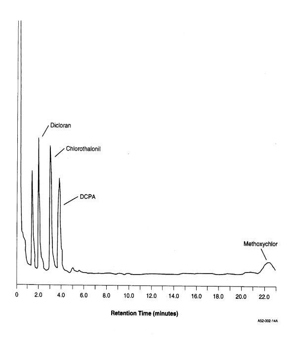
Figure 1. Gas Chromatogram of Chlorothalonil, DCPA, Dicloran, and Methoxychlor in a Wastewater Extract (Column 1)
