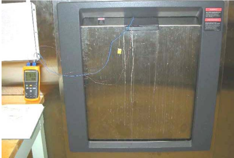
Figure 6. Autoclave door closed, with thermocouples passing through the top door seal.
