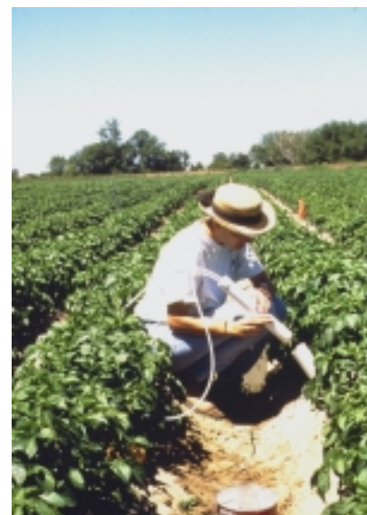
Lysimeter installation in potato crops (Eastern Snake River Plain, Idaho).
