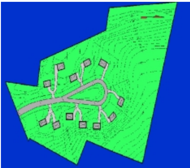
Treatment watershed site plan includes construction BMPs, shared driveways, pervious pavement and bioretention gardens (Jordan Cove, Connecticut).
