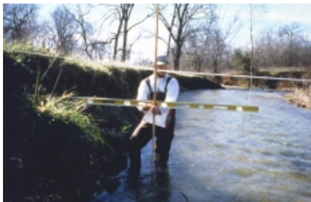
Measuring streambank erosion (Peach eater Creek, Oklahoma).
