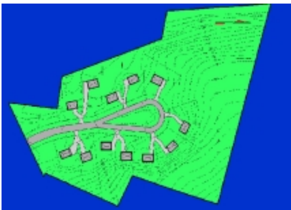
Treatment watershed site plan includes construction BMPs, shared driveways, pervious pavement and bioretention gardens (Jordan Cove, Connecticut).
