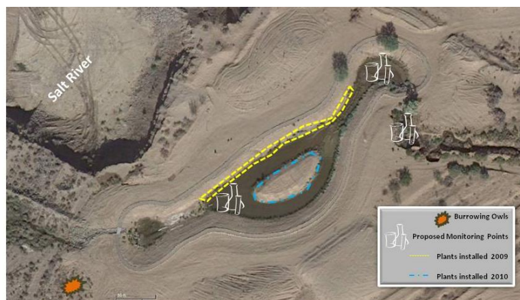
FIGURE 2.8 shows the Lehi Wetland sampling and monitoring locations as well as some planting installations.
