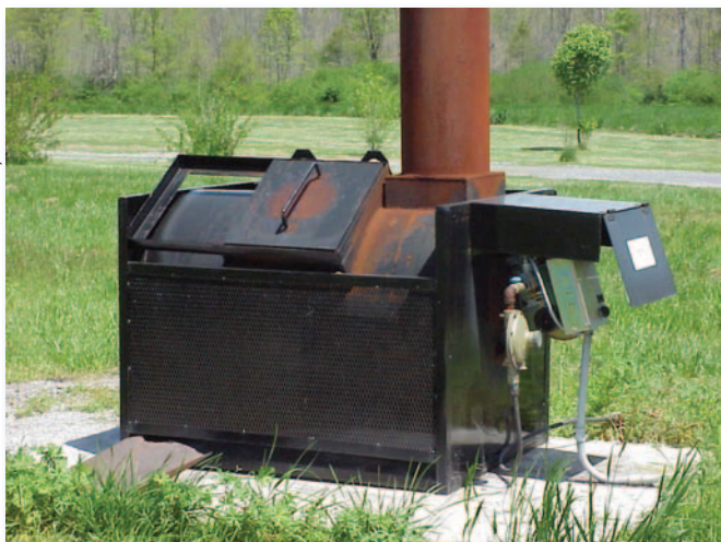
Figure 2. Ochlockonee River watershed poultry producers installed poultry incinerators such as this one.
