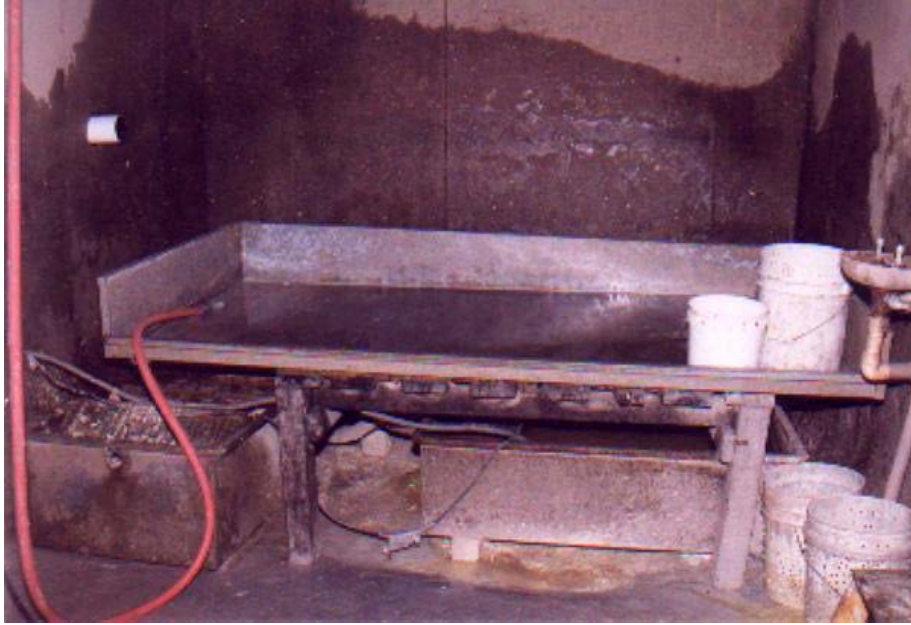
Figure_Apx D-2 Typical Water Wash Booth Used to Wash Stripper and Coating Residue from Furniture (IRTA, 2006)
