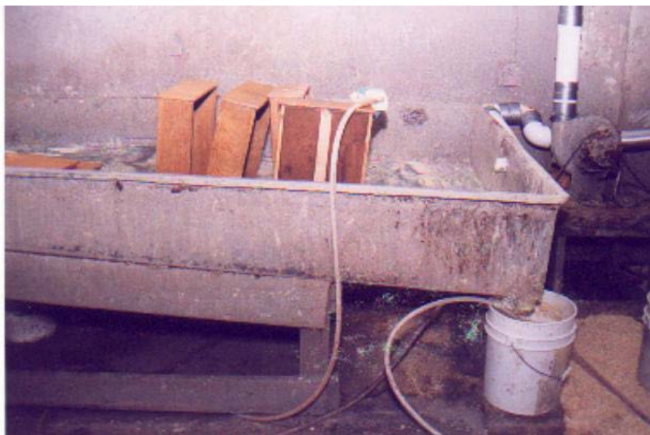
Figure_Apx D-1 Typical Flow Tray for Applying Stripper to Furniture (IRTA, 2006)
