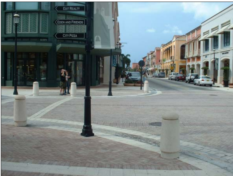
Figure 10.17 Use of contrasting material and bollards to delineate the pedestrian and vehicle areas. Source: Kimley-Horn and Associates Inc.
