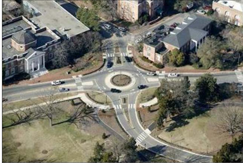
Figure 10.12 Typical layout of a single lane modern roundabout. Source: Kimley-Horn and Associates Inc.
