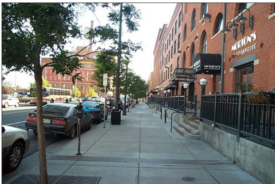
Figure 8.9 A combination of on-street parking, furnishings zone and wide pedestrian throughway provides ample buffer. Source: Kimley-Horn and Associates Inc.
