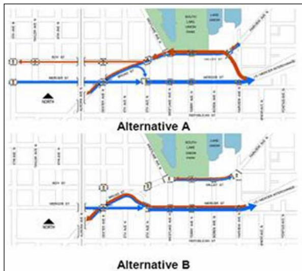
Figure 3.6 Corridor planning involves the consideration of trade-offs between alternatives. In this example different alignments and reconfiguration of streets are evaluated and compared. Source: City of Seattle, CHM2HILL, South Lake Union Transportation Study, Mercer Corridor Project.
