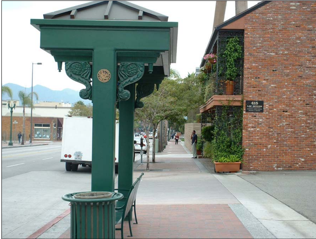
Figure 8.6 Utility poles and other fixtures should not interfere with the pedestrian throughway. This example shows a bus shelter and other street furniture properly located in the furnishings zone. Source: Kimley-Horn and Associates Inc.
