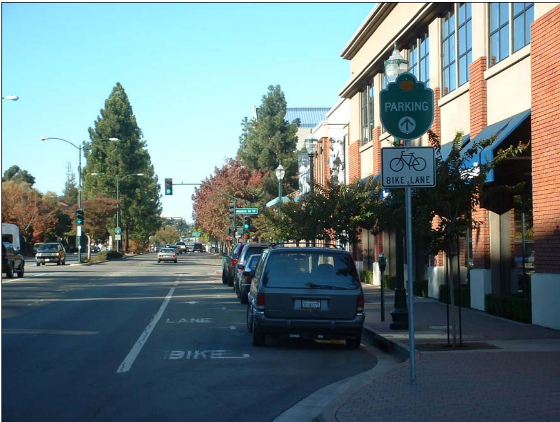
Figure 9.9 Bicycle lane adjacent to parking. Source: Kimley-Horn and Associates Inc.
