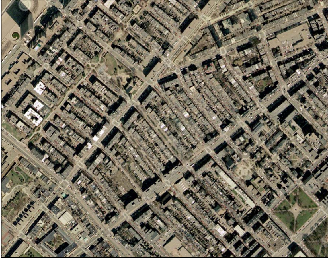
Figure 3.2 Example of a traditional network. Source: Data available from U.S. Geological Survey, EROS Data Center, Sioux Falls, SD.
