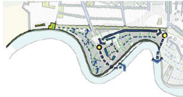
4 Sub-basin Redirected Discharge Optimizes Current Drainage System
