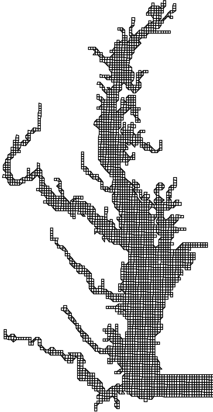
Figure B34. Physical and computational domain grid of the Chesapeake Bay. Grid spacing is approximately 1850 meters.
