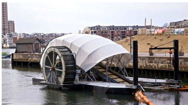
The Inner Harbor Water Wheel intercepts trash floating in a Baltimore, Maryland river before it can enter Baltimore’s Inner Harbor.
