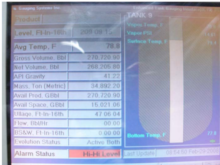
Photo 3 Tank 9 ATG on Feb 29th 2008 at 8:54 am (note level is 209' 9 and 15/16 th )
