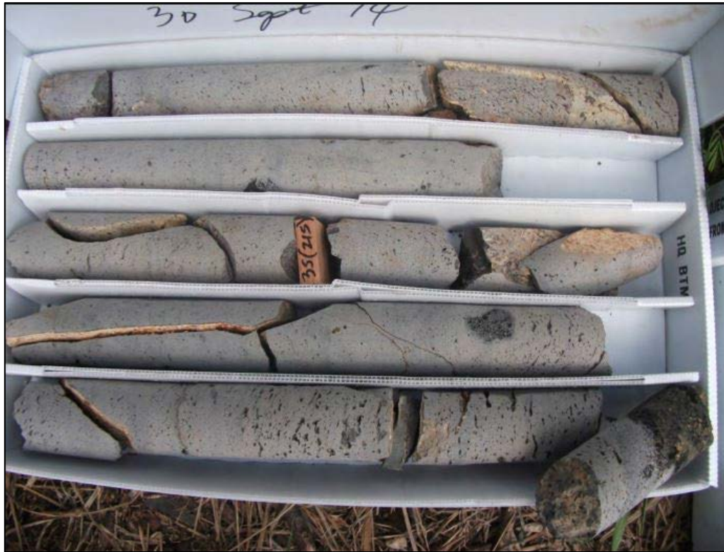
Photo 9: Boring at RHMW07 (surface elevation = 216.53 ft msl); core interval 210–220 ft bgs (-3.5–6.5 ft msl). Source: DON (2015b).
