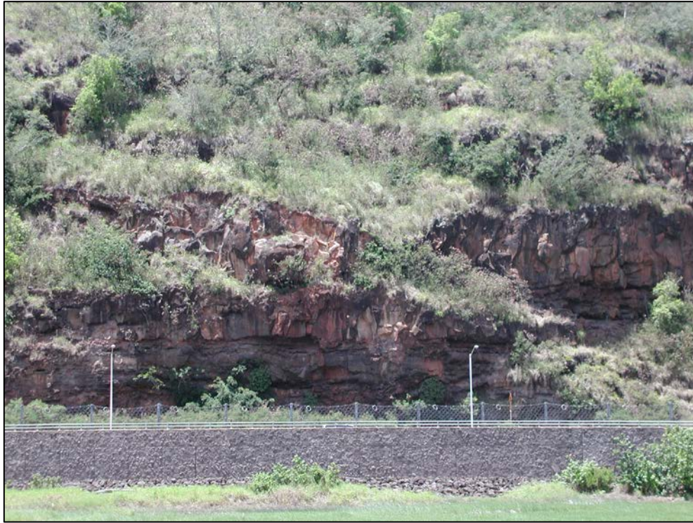
Photo 3: Thick massive a'ā flows exposed in outcrop on steep hillside; note widely spaced cooling joints and absence of open fractures in cores of flows. Photograph by Jack Kronen, AECOM, June 2005.
