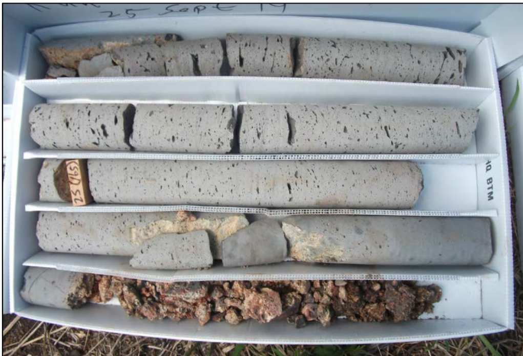
Photo 8: Boring at RHMW07 (surface elevation = 216.53 ft msl); core interval 160–170 ft bgs (46.5–56.5 ft msl). Source: DON (2015b).
