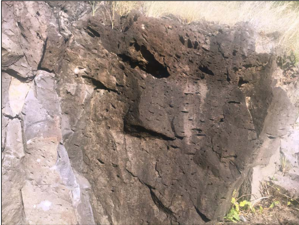
Photo 5: Closeup of massive a'ā core in outcrop; note stretched vesicles and absence of open fractures. Photograph by Jack Kronen, AECOM, January 2016.
