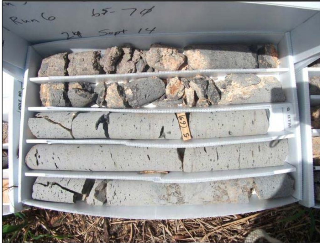
Photo 7: Boring at RHMW07 (surface elevation = 216.53 ft msl); core interval 60–70 ft bgs (146.5–156.5 ft msl). Source: DON (2015b).
