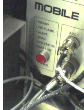
Heated Line Controller MPS Power/Air Filter SEMTECH DS Power Switch
