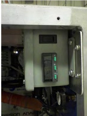
Heated Line Controller MPS Power/Air Filter SEMTECH DS Power Switch
