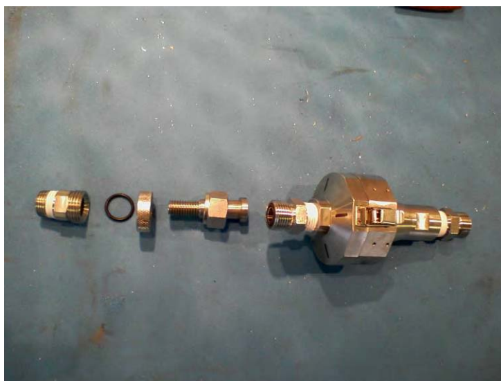
47 mm filter cup assembly
