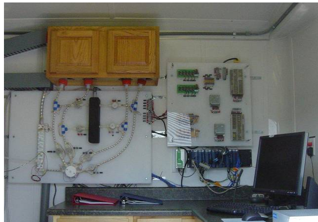
Figure 6. Photograph of the positive-pressure gas sampling system used in the study.
