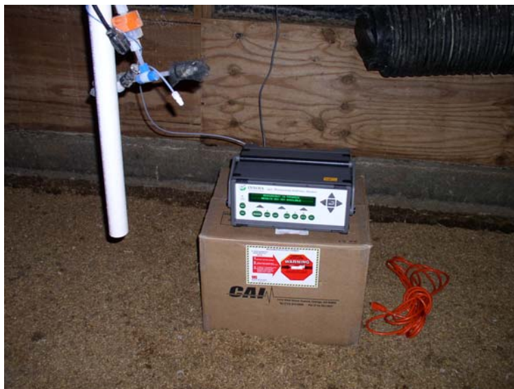
Figure 14. One of the three in-house INNOVA analyzers used to compare readings to its counterpart inside the MAEMU.
