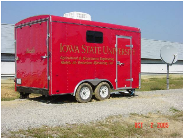
Figure 4. Environmentally-controlled Mobile Air Emissions Monitoring Units (MAEMU).
