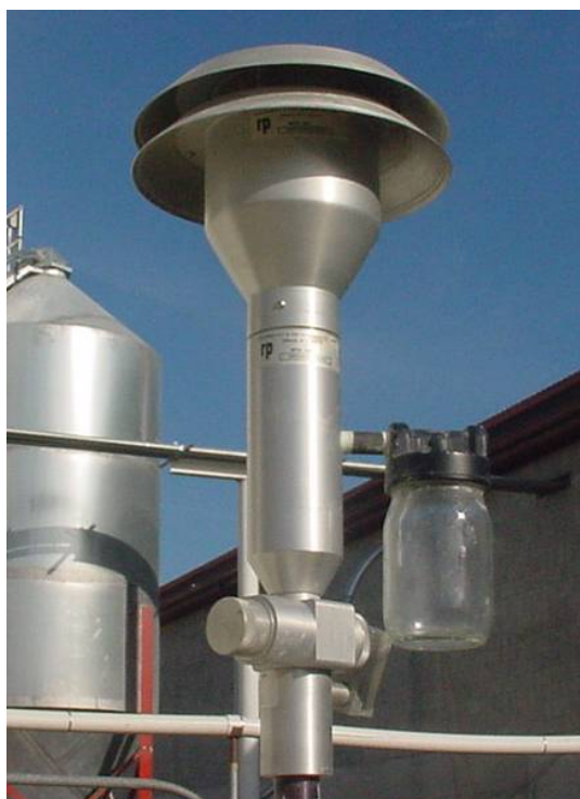
Figure 2. TEOM PM 10 and PM 2.5 inlets (left), and a closeup of the PM 2.5 inlet (right, photo provided by TEC).
