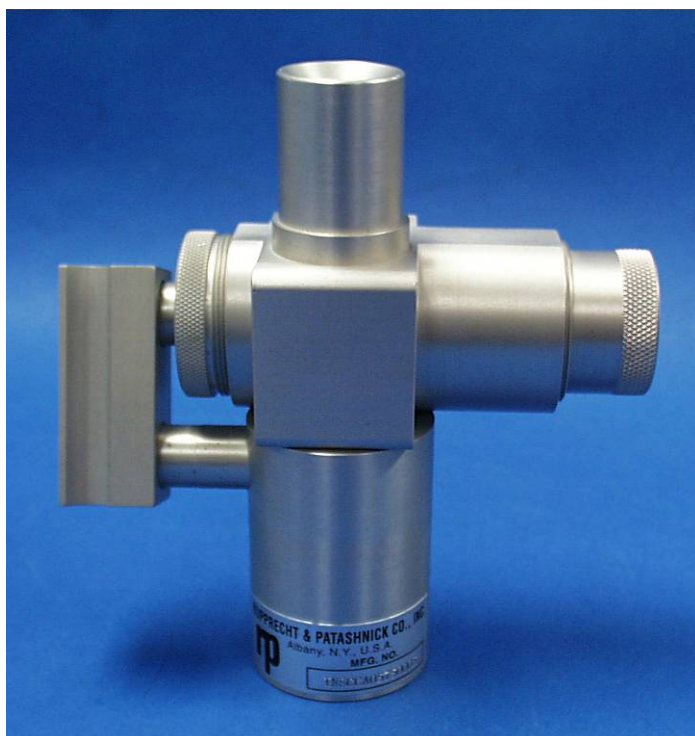
Figure 2. TEOM PM 10 and PM 2.5 inlets (left), and a closeup of the PM 2.5 inlet (right, photo provided by TEC).
