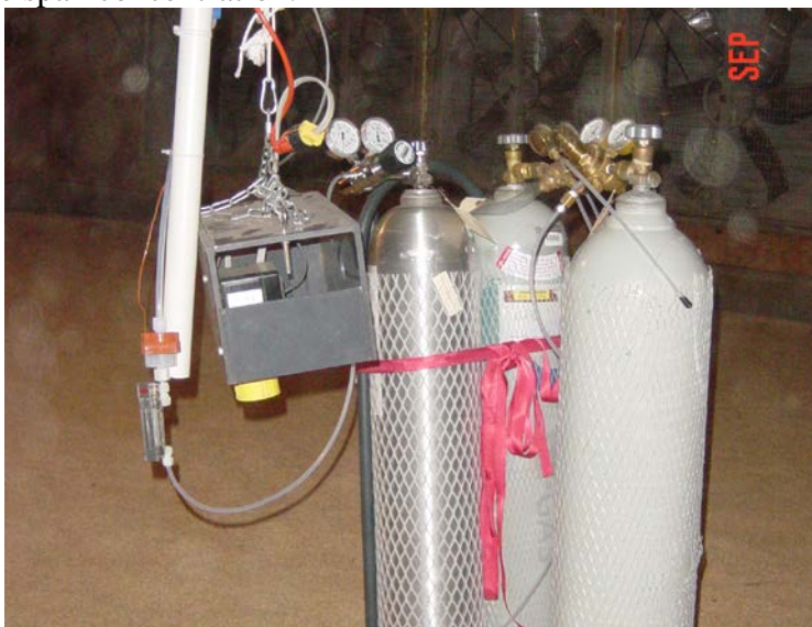
Figure 15.1. Picture of span gas injection from sampling points.
