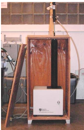
Figure 1. TEOM sensor unit in a custom-made enclosure.
