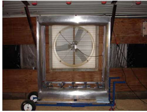
Fan calibration by FANS unit
