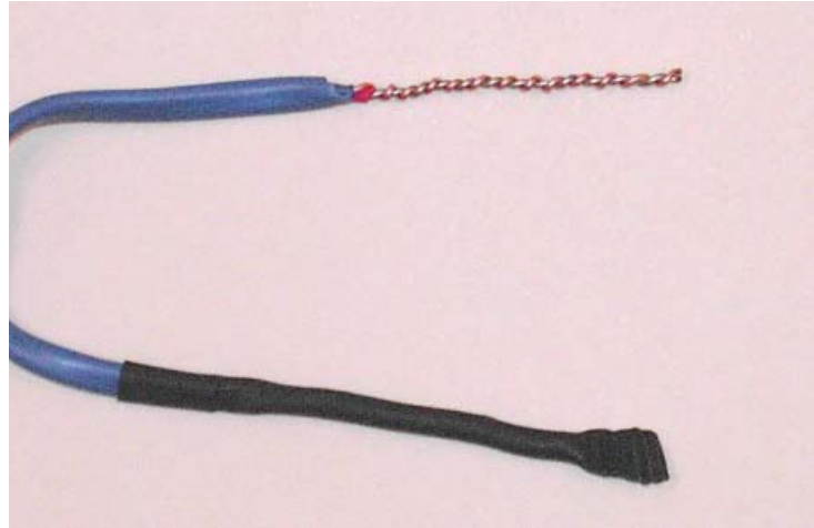
Figure 1. Steps in thermocouple fabrication. Shown are the twisted wire pair after cutting (Step 9.1.2) and the fully-attached shrink wrap (Step 9.1.3).
