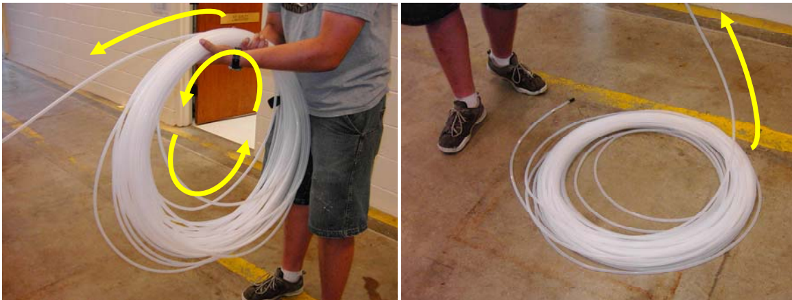
Figure 1. The correct (left) and incorrect (right) way to uncoil Teflon tubing when a feeder device is not used.
