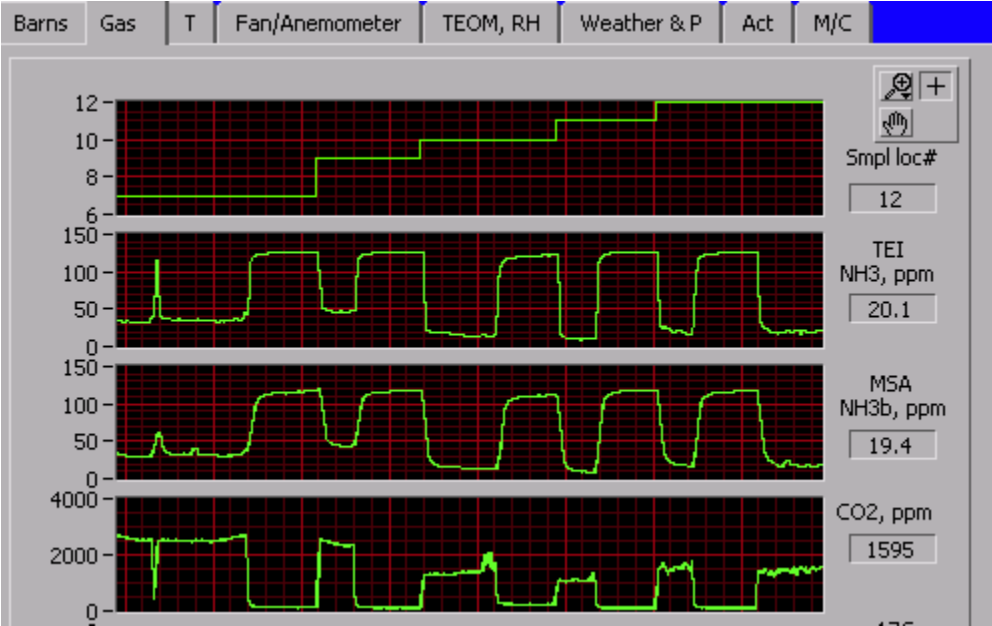
Figure 9. Responses of the two ammonia gas analyzers to a test using ammonia-filled bags at five sampling locations.
