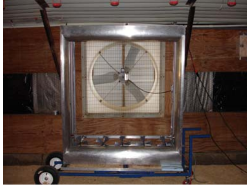
Fan calibration by FANS unit
