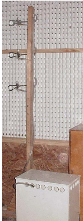
Figure 3. A TSP sampling system (three filter cassettes, tubing, and the white sampling pump box on the left) with sampling filters and tubes attached to a sturdy 2x4 post.
