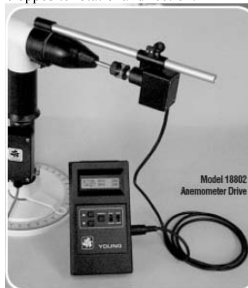
Figure 4. Model 18802 Anemometer Drive (R.M. Young 2000).
