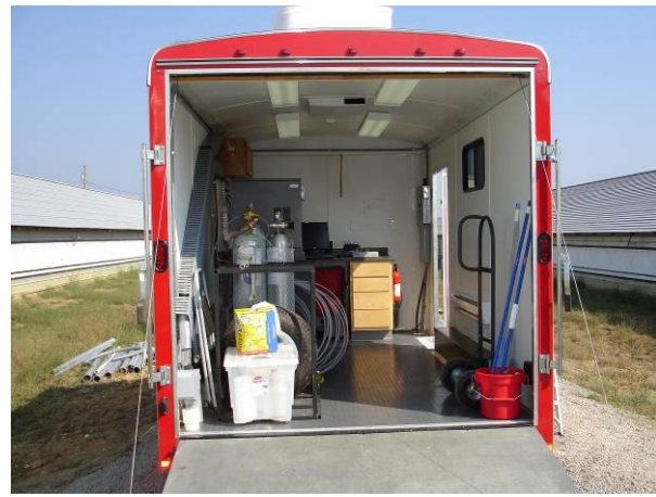
Figure 6.4. Environmentally controlled Mobile Air Emissions Monitoring Units (MAEMU).
