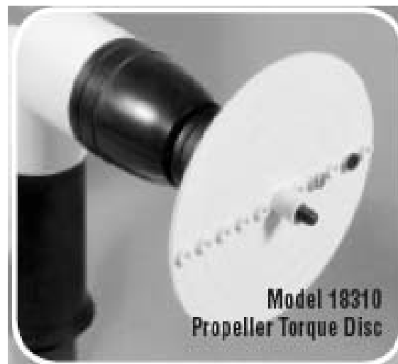
Figure 3. Model 18310 Impeller Torque Disc (R.M. Young 2000).
