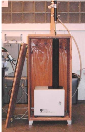
Figure 1. TEOM sensor unit in a custom-made enclosure.
