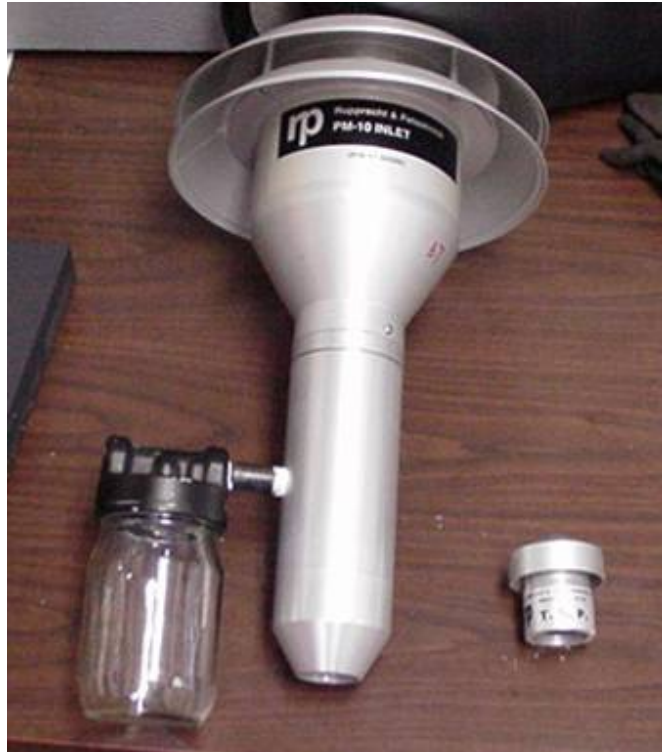
Figure 3. TEOM PM 10 (left) and TSP inlets (right).
