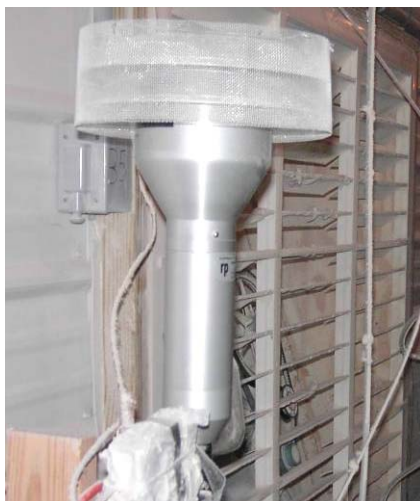
Figure 4. TEOM PM 10 inlets with external screens installed.
