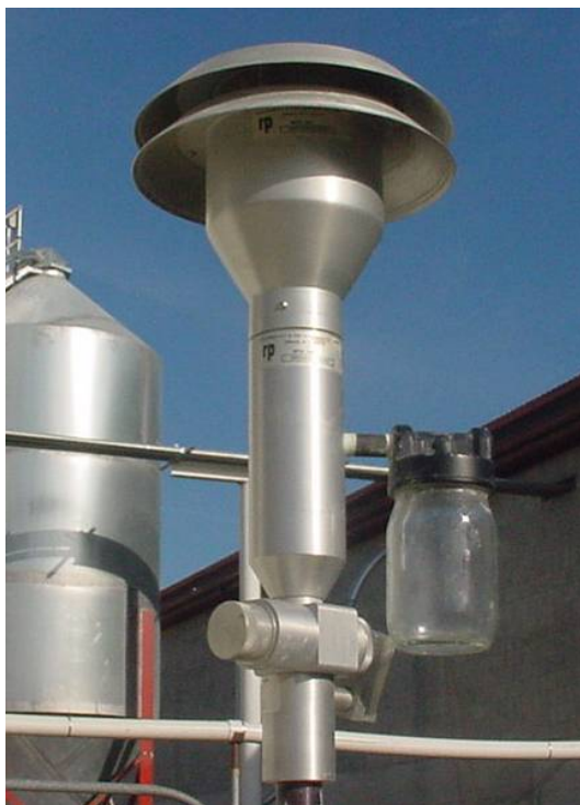
Figure 2. TEOM PM 10 and PM 2.5 inlets (left), and a closeup of the PM 2.5 inlet (right, photo provided by TEC).
