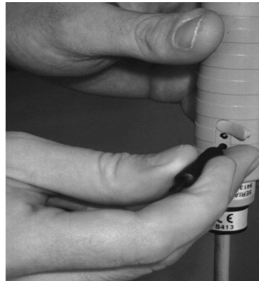
Figure 2. Potentiometer adjustment location on the HMP45C.
