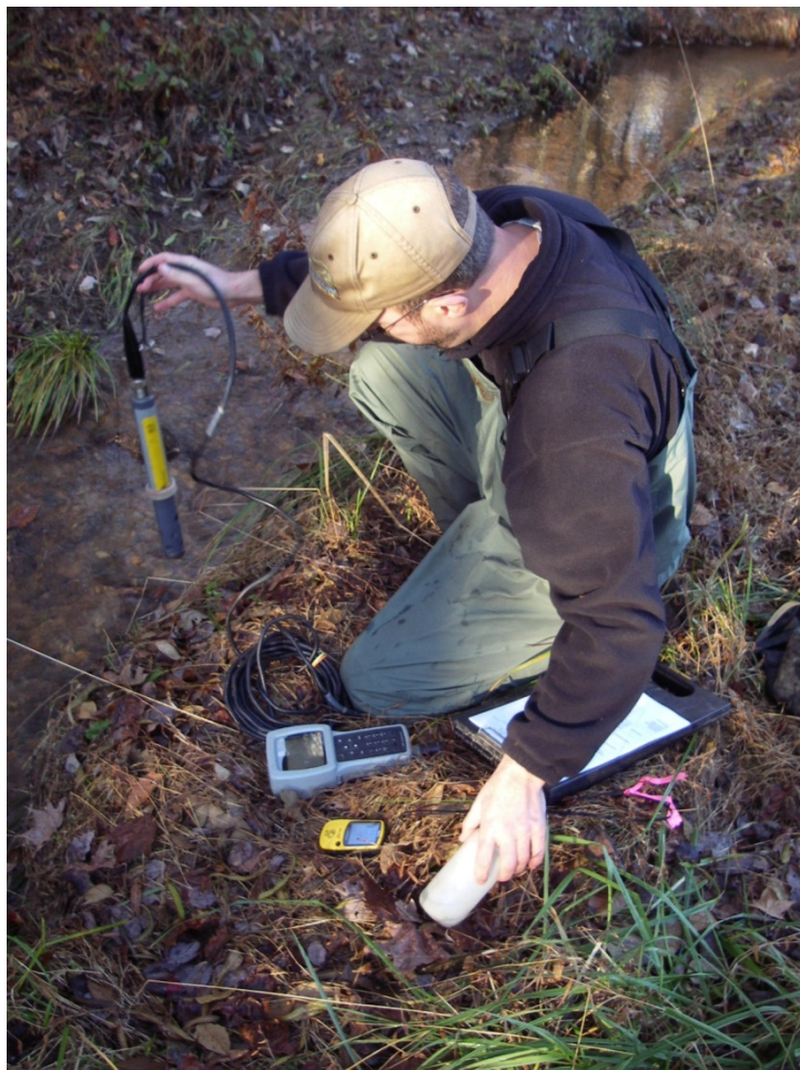
Figure 3-35. Measuring dissolved oxygen, specific conductance, pH, and water temperature using a hand-held probe
