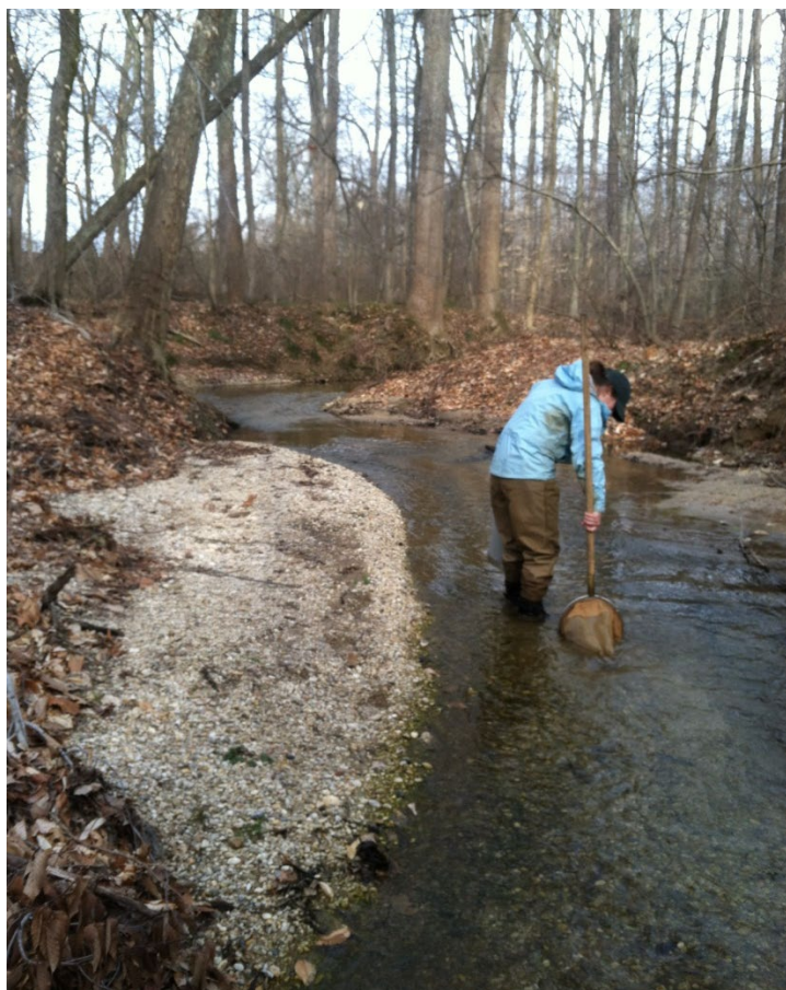
Figure 3-43. Using a D-frame net to sample a gravel bottom stream for benthic macroinvertebrates
