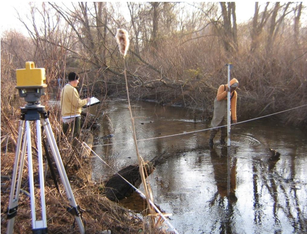
Figure 3-9. Measuring the cross-section profile of a stream channel
