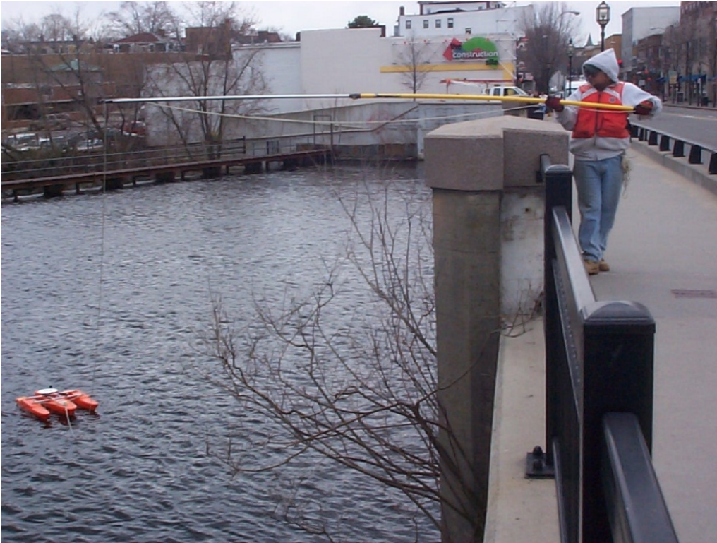
Figure 3-10. Measuring discharge from bridge using an ADCP (acoustic Doppler current profiler) unit (USGS 2007)
