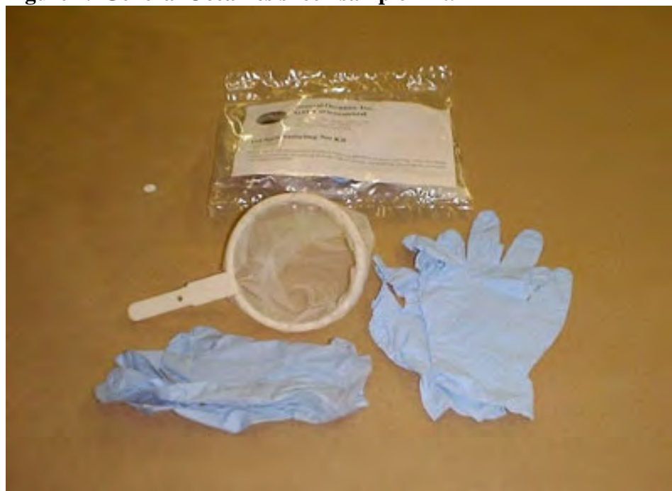
Figure 1. General Oceanics sheen sampler kit.
