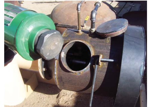
Internal View of Auxiliary Burner Unit and Venturi. Photo Courtesy of EnCana.
