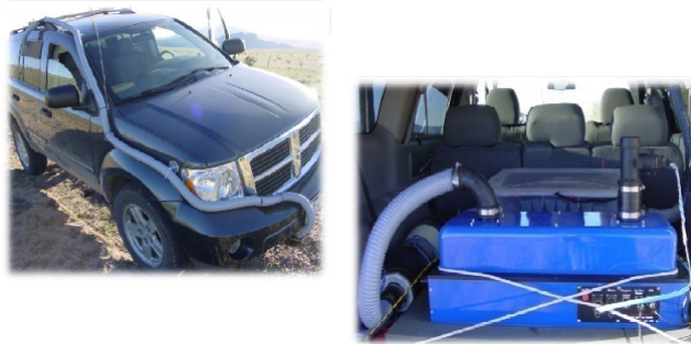
Exhibit 3: Apogee Truck-Mounted Leak Detection System ( www.apogee-sci.com/Forms/ApogeeLDS012610v1.pdf )
