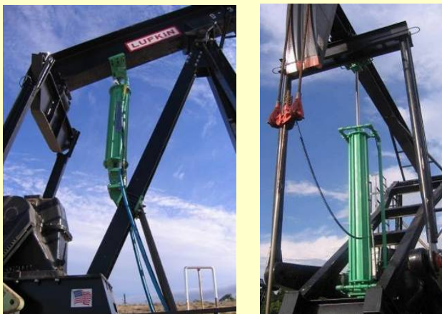
Exhibit 2: Two Beam Gas Compressors™ each utilizing the mechanical energy of a pumpjack to pull gas from the casing and discharge it into a flowline (Source: Permian Production Equipment, Inc.).
