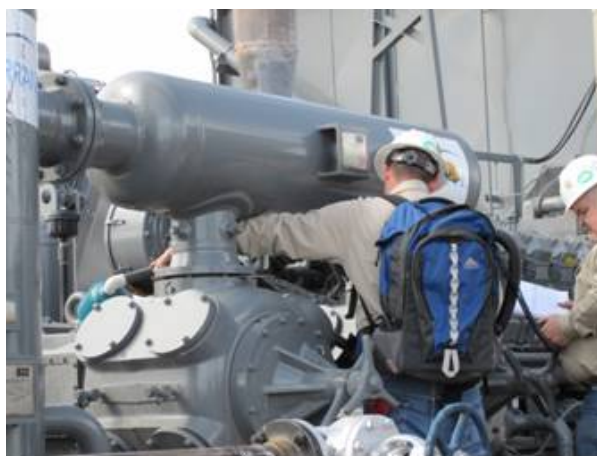
Exhibit 2: Measurement experts quantifying a methane emissions source with the Hi Flow Sampler at Pleasant Valley station during the Natural Gas STAR workshop site visit.
