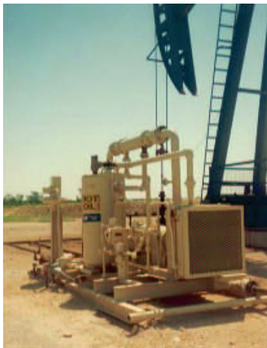
Exhibit 1: A skid-mounted compressor package recovering casinghead gas at a wellhead (Source: Hy-Bon Engineering).
