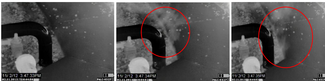
Figure 4. Photographic Sequence of a Natural Gas Fugitive Emission from an Underground Line.
