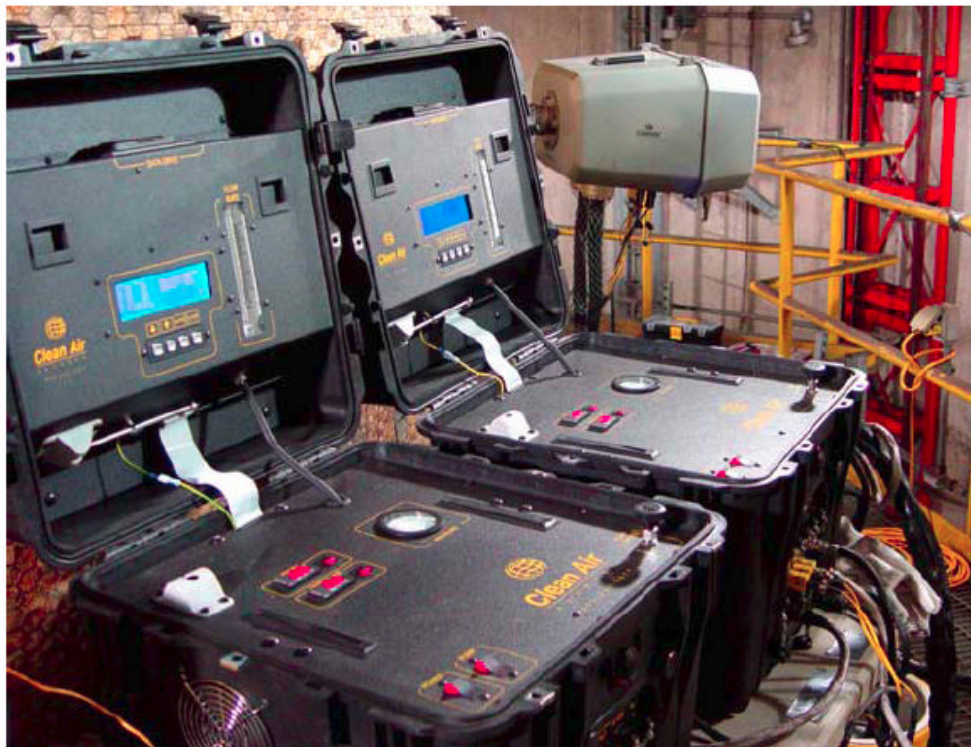
Figure 4-41: Portable Sampling System in Use at Armstrong Unit 2 Stack
