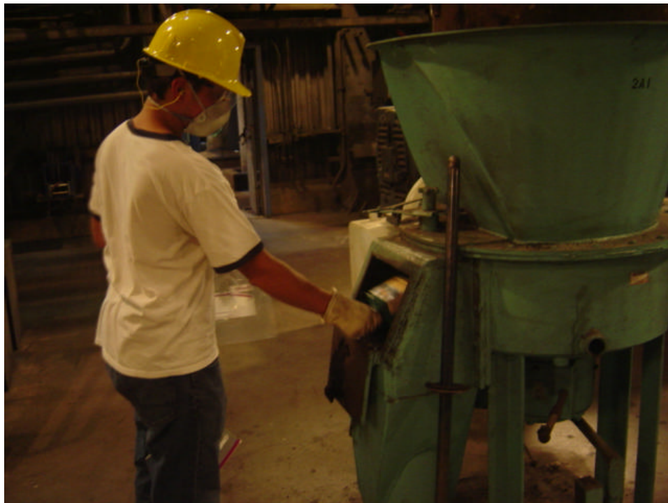
Figure 3-2: Collection of Coal Samples from Mill Feeders
