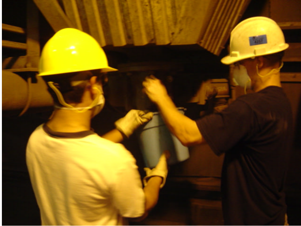
Figure 3-3: Collection of Ash Samples from the ESP Hoppers
