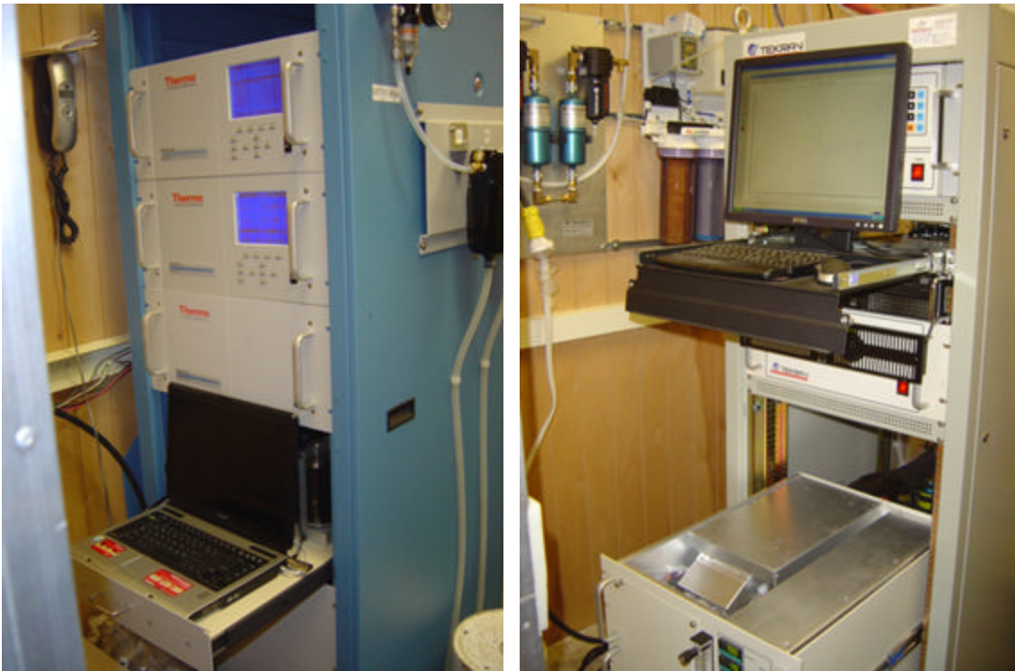
Figure 3-15: Thermo Electron and Tekran CMMs Located in CEM Shelters at Armstrong
