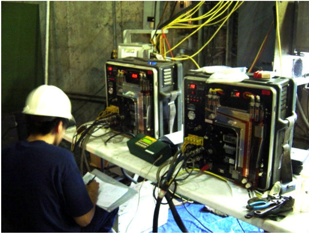
Figure 4-9: Manual Adjustments to Maintain Isokinetic Sampling
