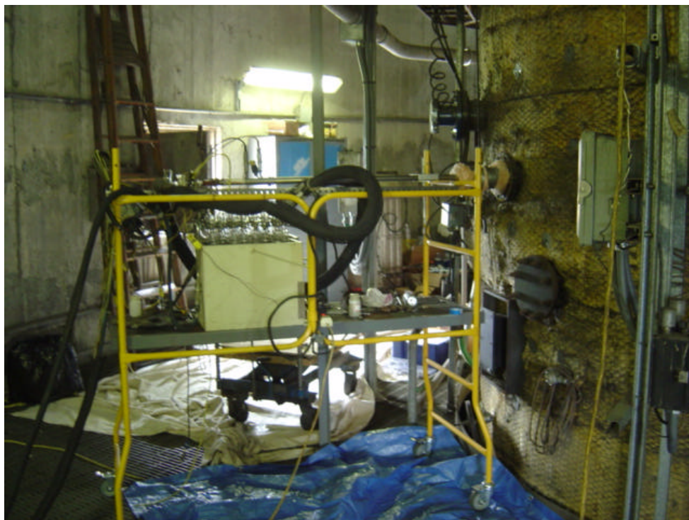
Figure 4-6: Paired OHM Sampling Train at Armstrong
