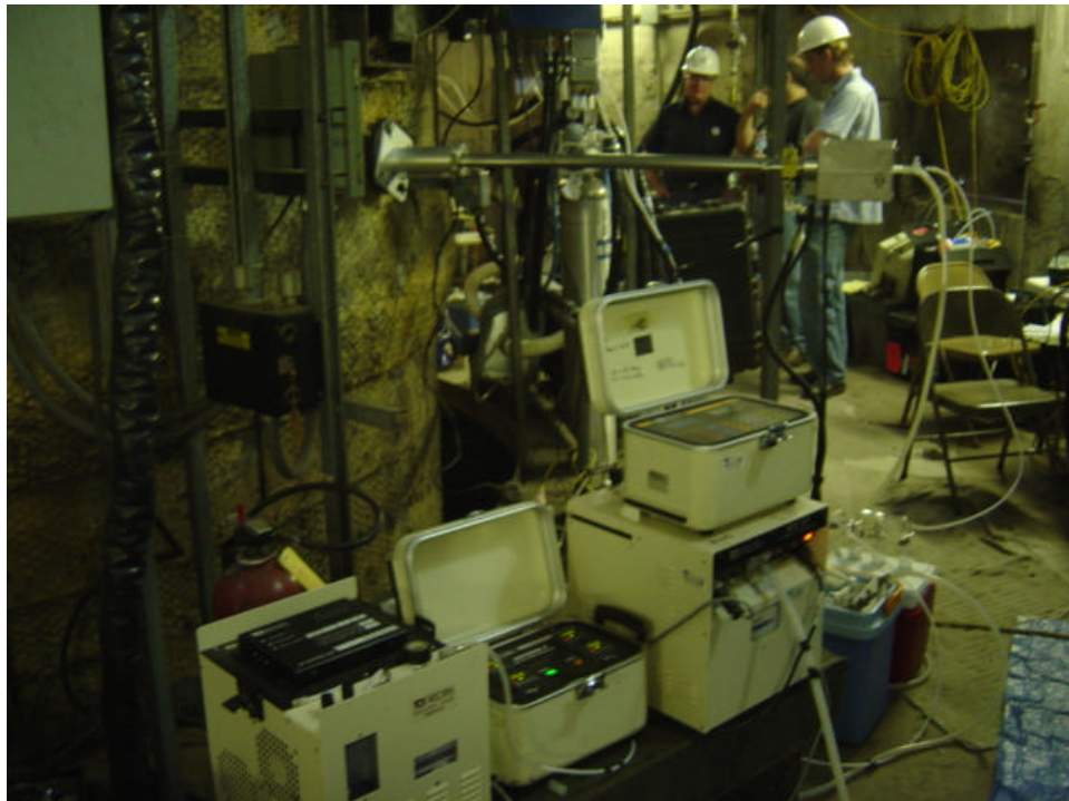
Figure 4-18: EU Sampling System at Armstrong
