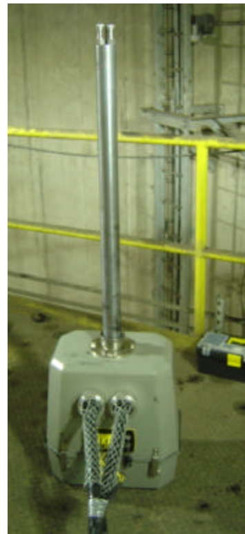
Figure 3-12: CleanAir/CONSOL Equipment for Hg Measurement According to Appendix K Sorbent Trap Method, Located on the 4 th CEM Platform
