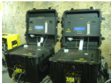
Figure 3-12: CleanAir/CONSOL Equipment for Hg Measurement According to Appendix K Sorbent Trap Method, Located on the 4 th CEM Platform
