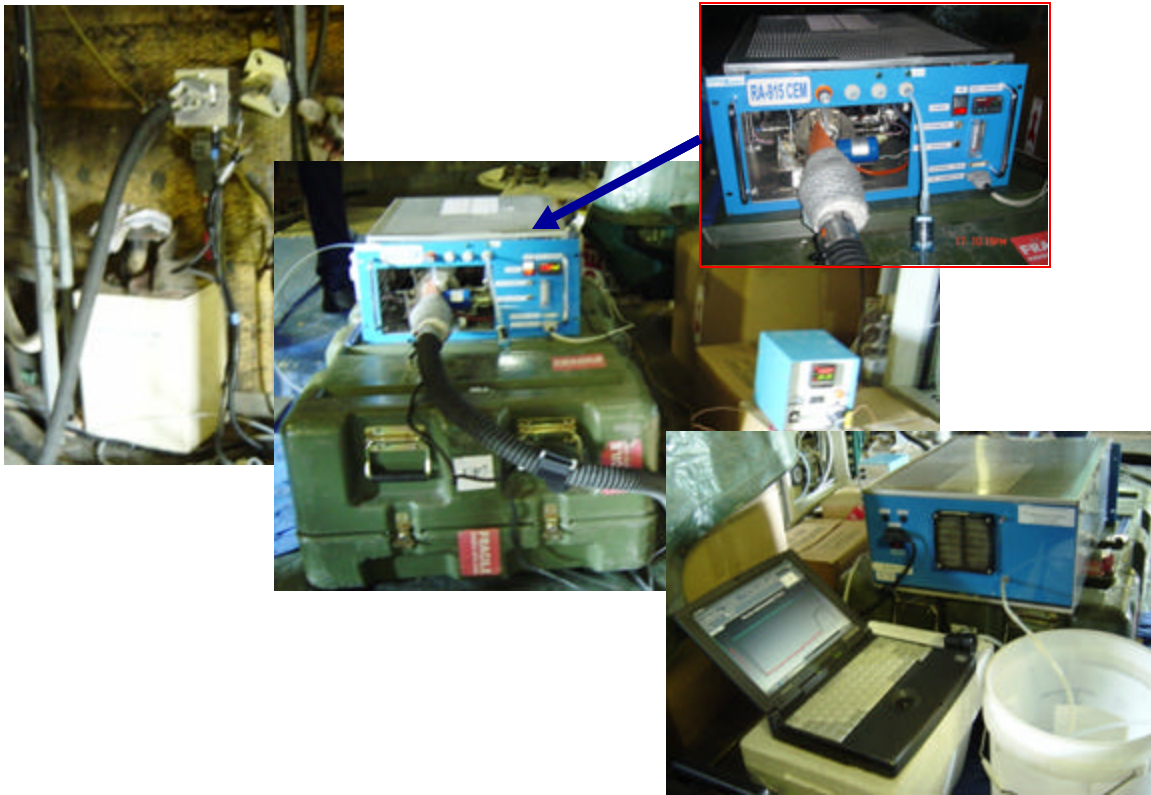
Figure 6-2: Sampling Train for Hg T Traverse: System Components
