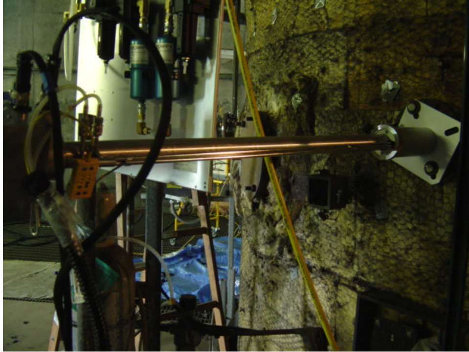
Figure 4-17: EU Sampling Probe Inserted In a Sample Port at Armstrong
