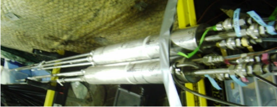
Figure 6-6: Fixed Array Sorbent Trap Probes Used at Armstrong
