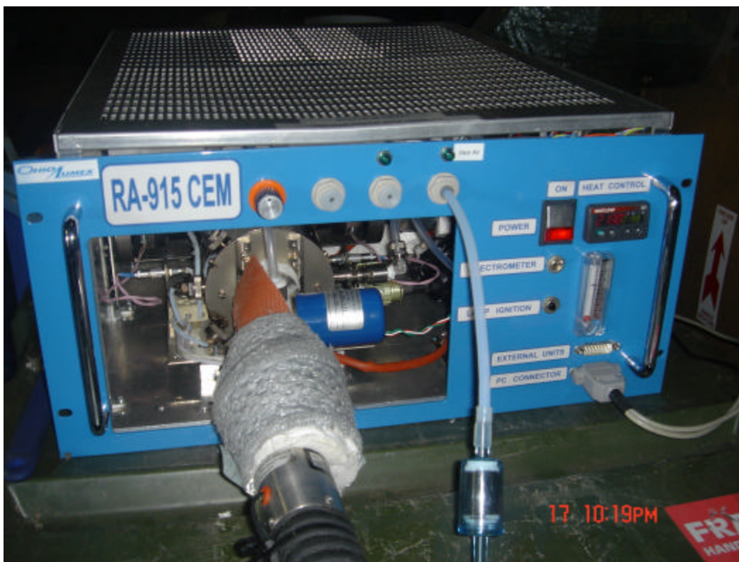
Figure 4-34: Ohio Lumex RA 915 CEM Used at Armstrong
