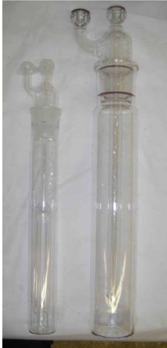
Figure 4-19: EU Impinger (left) In Comparison to the Smith Greenburg Impinger (right)
