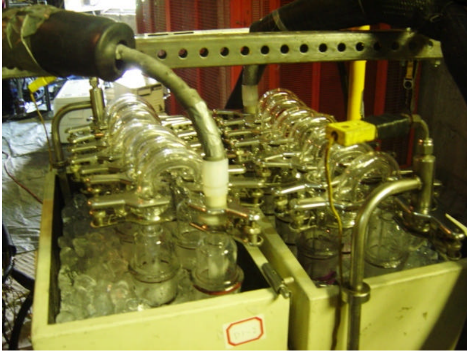
Figure 4-7: Impinger Boxes for Paired OHM Sampling Train
