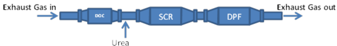
Figure III-3: SCR Upstream of DPF
