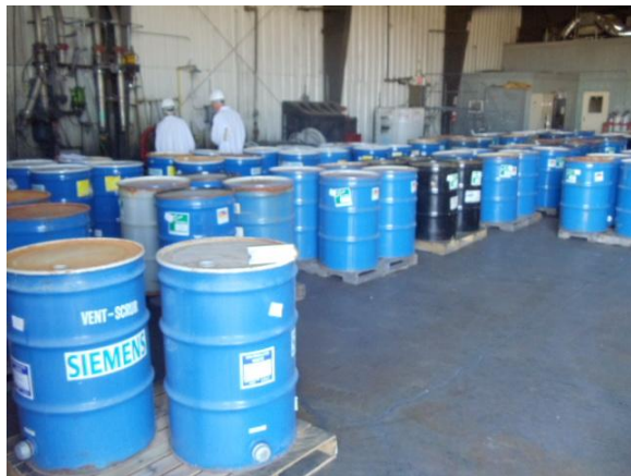
Photo #3: Numerous 55-gallon containers of spent carbon (26 hazardous waste storage containers; rest are nonhazardous) in the IS container storage area.
