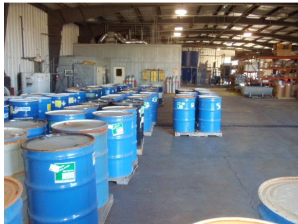
Photo #4: Another view of the 55-gallon spent carbon storage containers in the IS container storage area.
