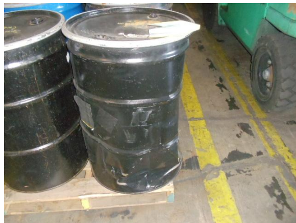
Photo #13: View of hazardous waste storage container on bottom right in Photo #11. The container is not in good condition (dented).
