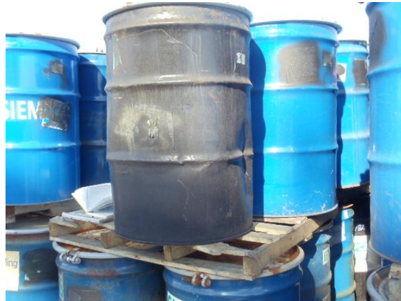
Photo #16: Facility personnel emptied sludge from the dented container shown in Photo #13, triple rinsed the container, and placed it in the empty container storage area.
