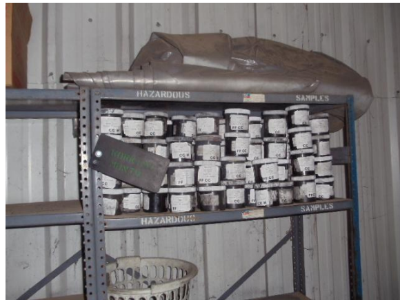
Photo #27: Hazardous spent carbon retain samples in the IS container storage area.
