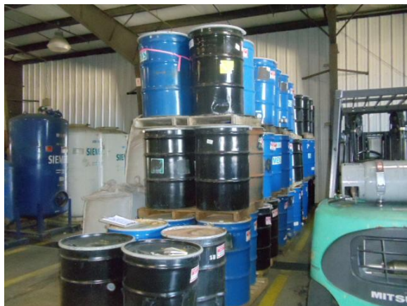
Photo #11: 76, 55-gallon hazardous waste storage containers holding filter press cake in IS container storage area.
