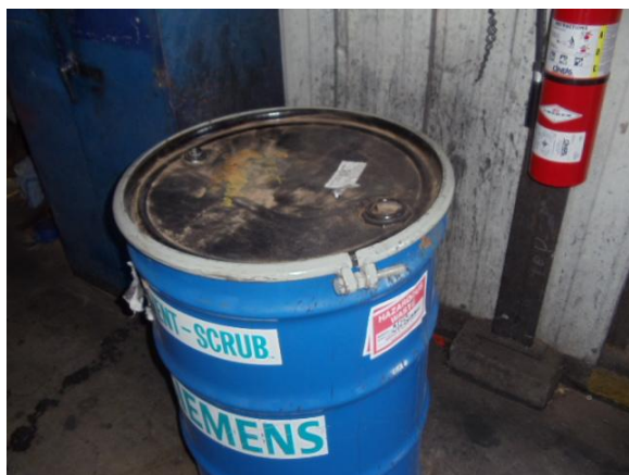
Photo #50: Satellite accumulation container shown in Photo #48 after facility representatives replaced the lid.
