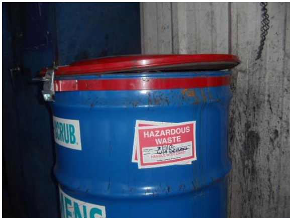
Photo #48: Warehouse Loading Area satellite accumulation container; lid is damaged and will not close.
