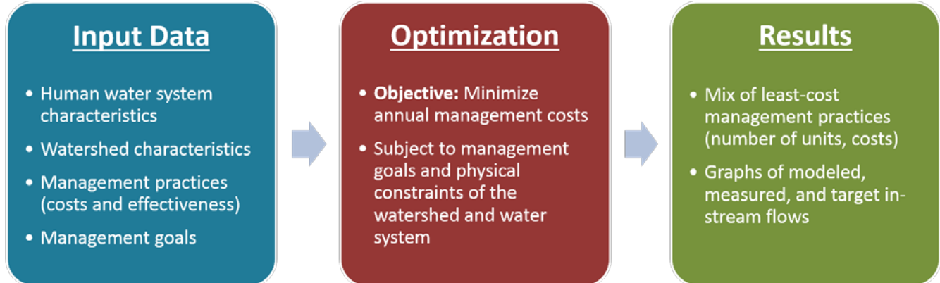
Figure 2. WMOST modeling process from user inputs through to results used to derive optimal solutions.
