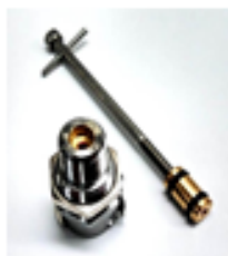
Modified CPC fitting and critical orifice installation tool
